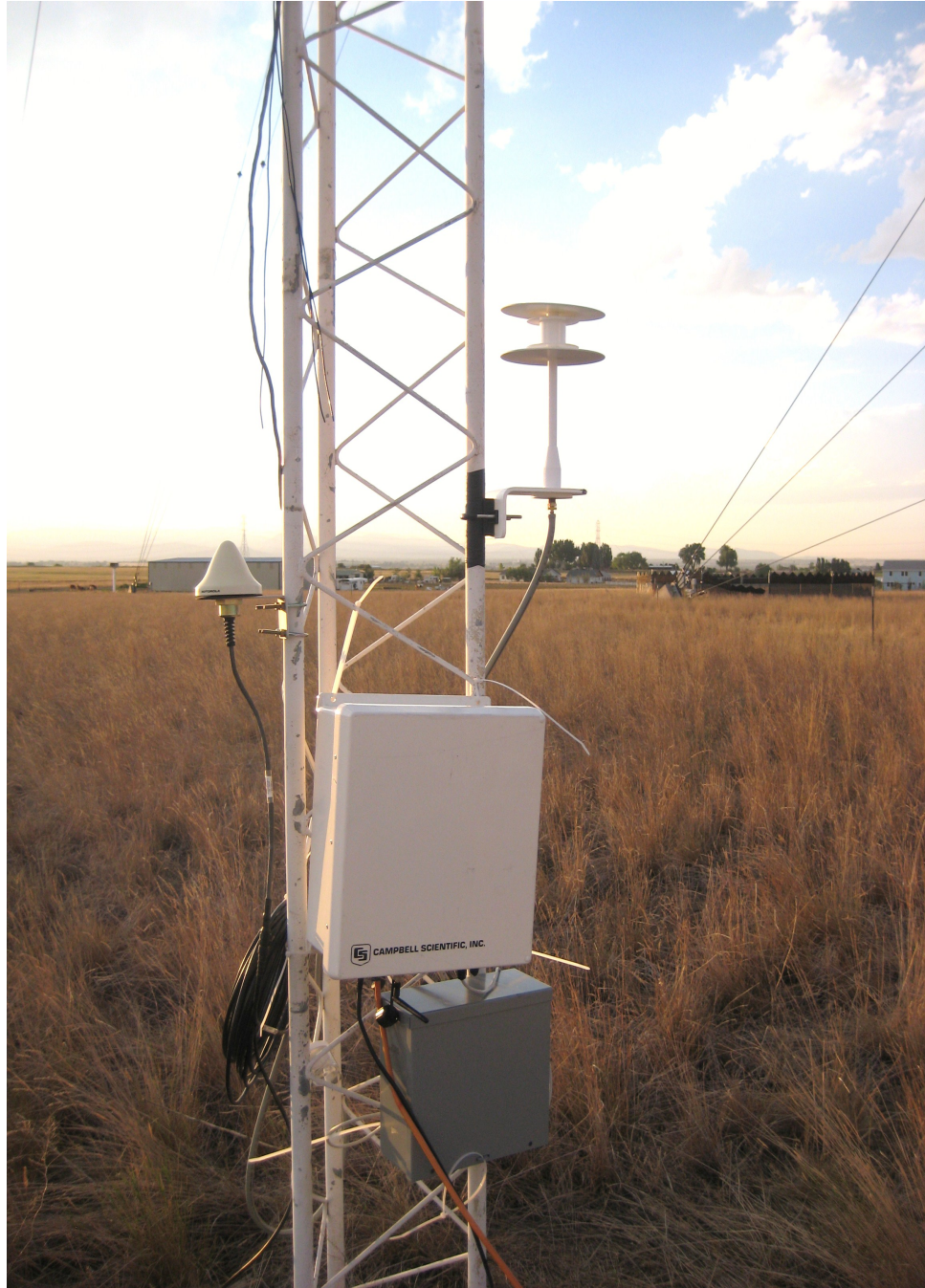
Figure 3.1. Data Logger in its protective enclosure by Campbell Scientific: The picture was taken during an experiment at the Boulder Atmospheric Observatory (BAO) near Erie, Colorado during Aug 2008. The DigiPort can be seen above the data logger on the right.
