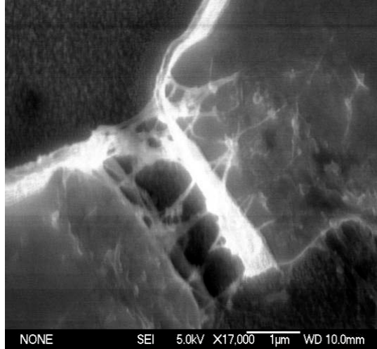
Figure 2.40 SEM images for devices 4A3. Complicated network of CNT bundles with big overlap with metal bridges the 1\mu\text{m} gap.
