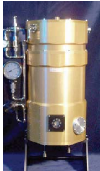
Figure 1.10 Conceptual model of a common bolometer device. Note that the thermal conductance G ( G_{th} ) is the main link for the device to dissipate the energy acquired from the incident power (left, from ref. [35]). Typical Si superconducting bolometer (right), spectral response from 2 - 3000 \mu m, operating temperature from 4.2 - 0.3K. The bolometer responds only to an AC signal within detector bandwidth.
