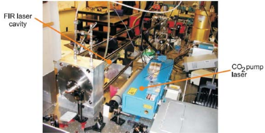
Fig. 2.34 CO 2 pumped FIR gas laser used as THz source.
