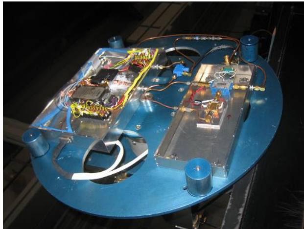
Figure 3.15. Two box setup mounted on the spinning portion of the antenna assembly.
