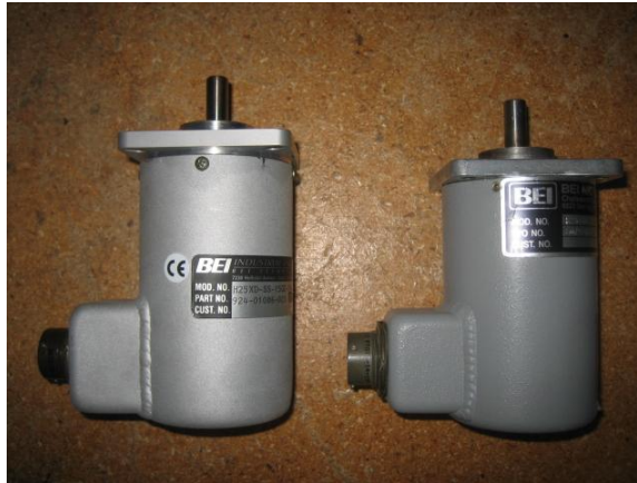
Figure 4.5. IWRAP 15 bit (New) and 10 bit (Old) BEI encoder system for the Ku-band antenna assembly.
