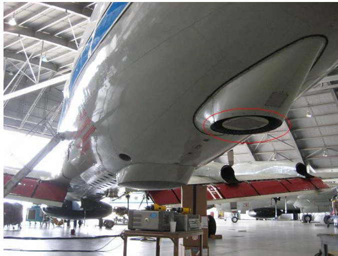
Figure 3.7. NOAA P3 Platform where the Ku-band antenna assembly is installed.
