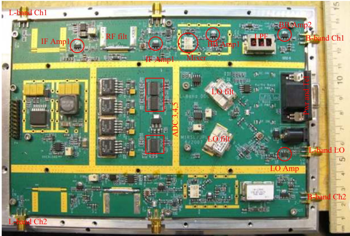
Figure 4.14. Picture of the L-band to baseband downconverter PCB
