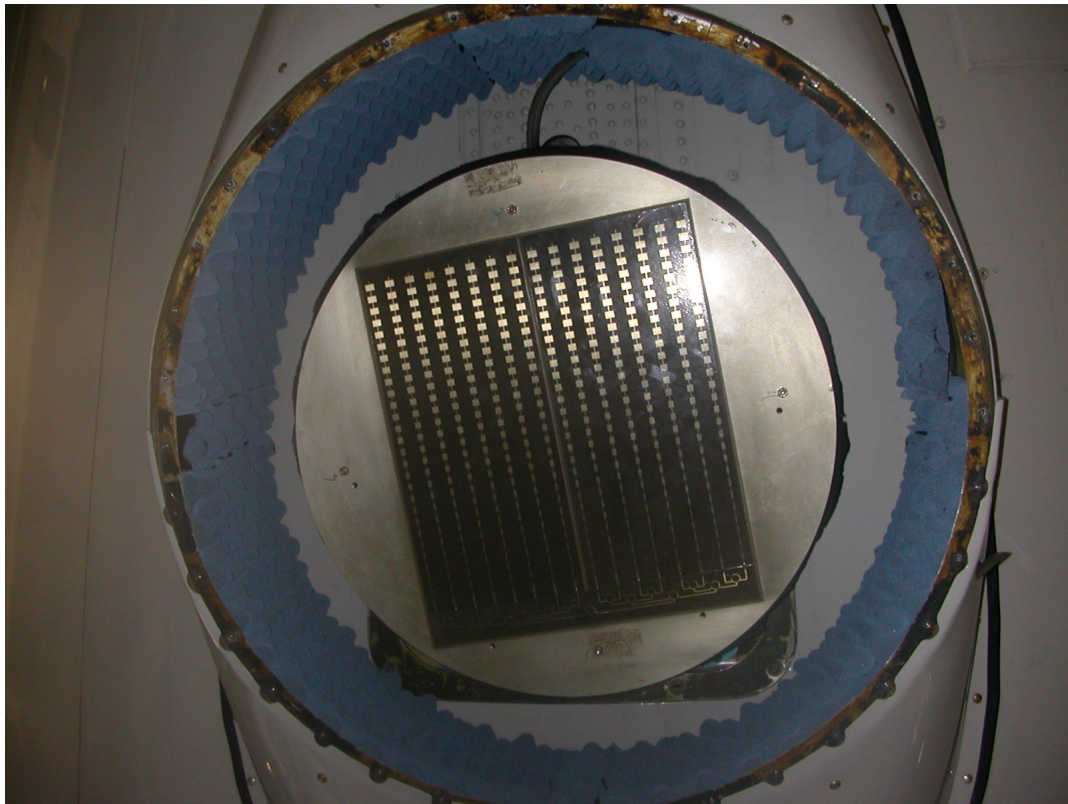
Figure 2.10. Mounted Ku-band single-polarization (vertical) antenna used for the 2008 hurricane season
