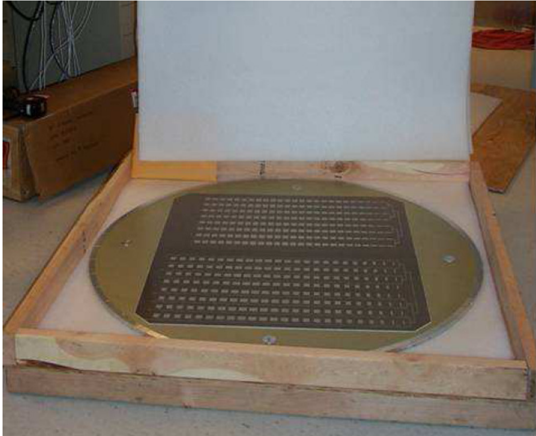
Figure 2.11. C-band dual-polarization antenna used for the 2008 hurricane season (only H-polarization was used)
