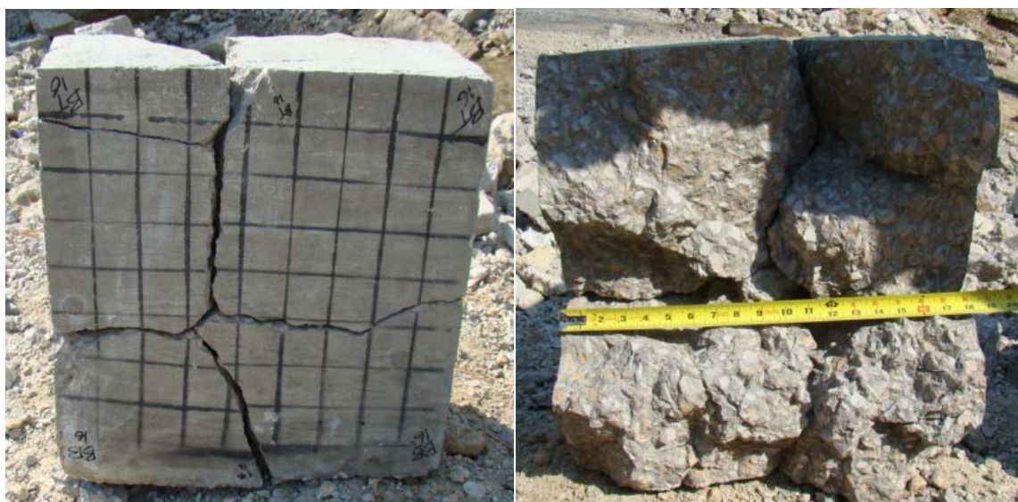
Figure 4.21: Block 16, back face and interior views after impact
