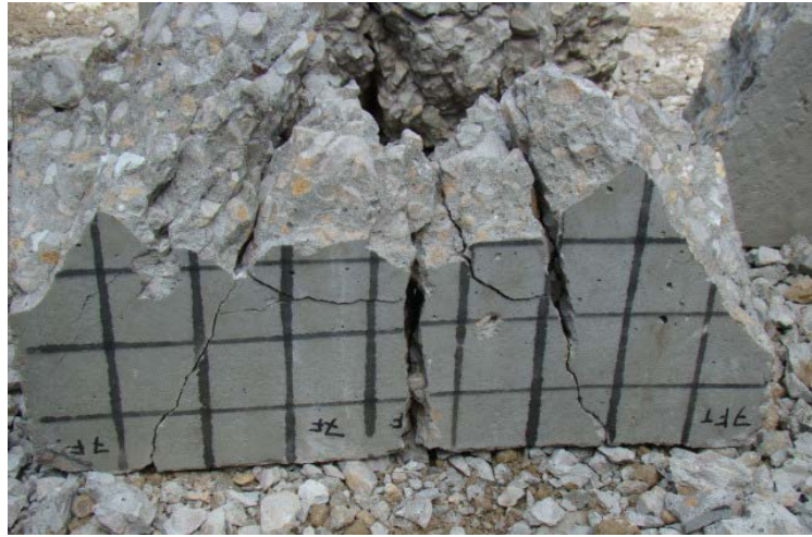
Figure 4.11: Block 7, front face pieces recovered after impact.
