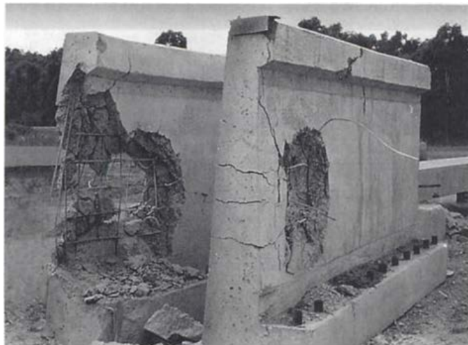
Figure 1.1: Reinforced concrete after EFP impact.(2)
