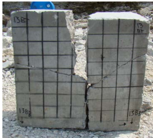
Figure 4.18: Block 13, back face after impact
