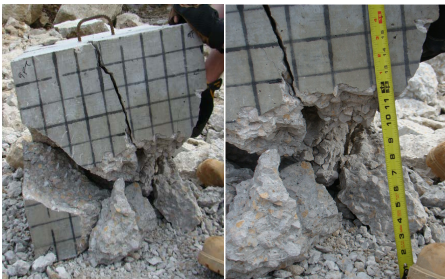
Figure 4.14: Block 9, front face after impact.
