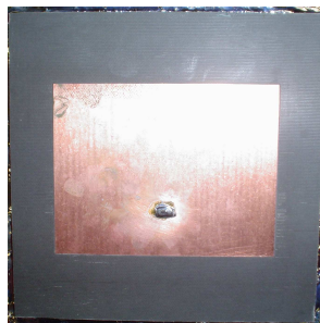
Figure 90 - Built transmit antenna for use in the far-field range.
