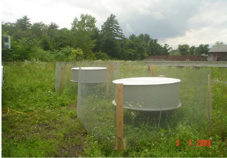
Figure 5.8. Shroud fence built around the Wind Profiler antennas
