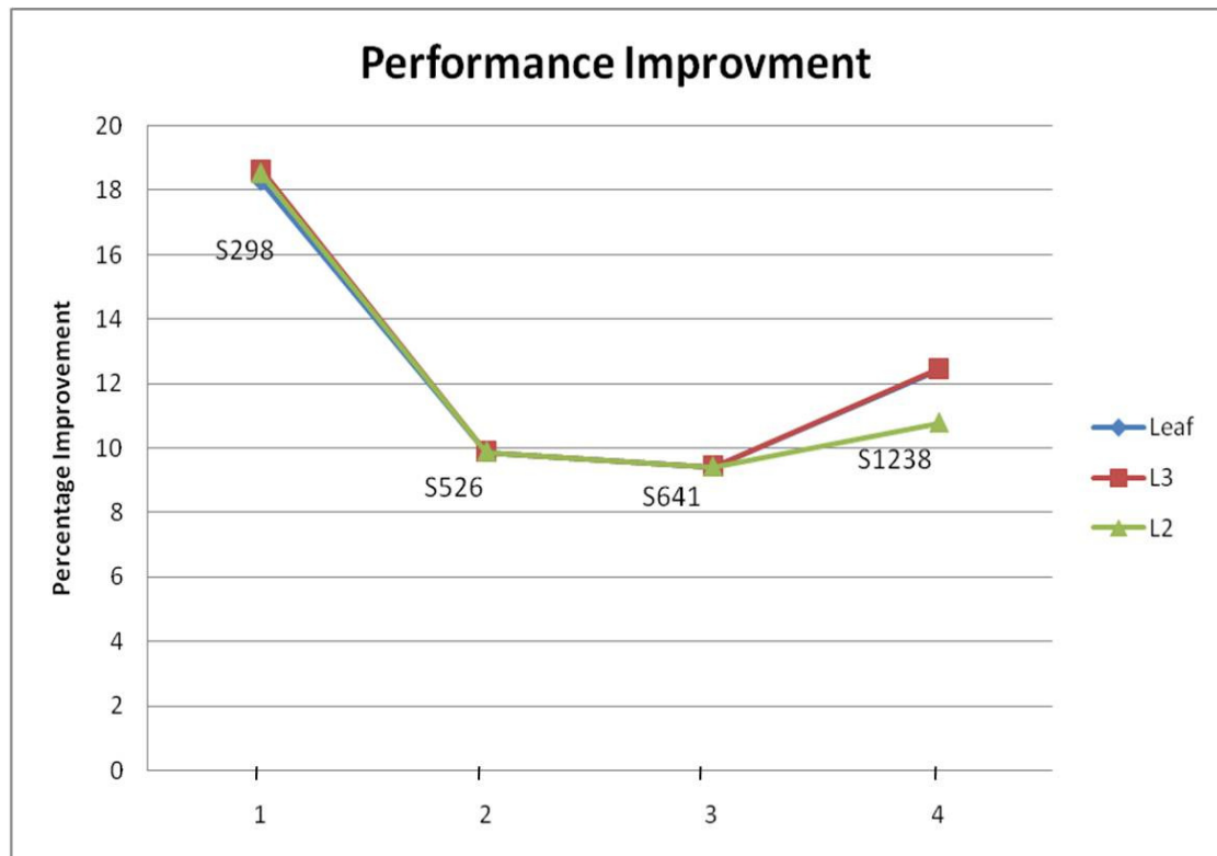
Figure 34: Performance improvement with clock tuning for ISCAS 89 benchmark circuits
