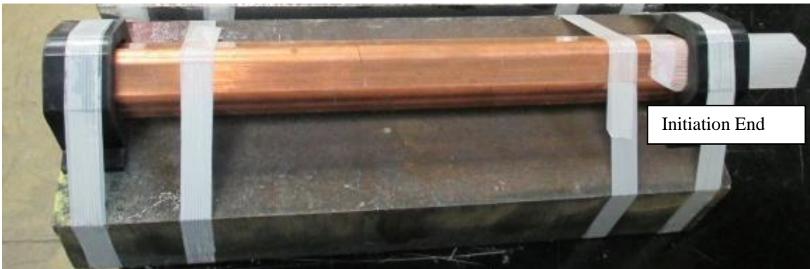
Figure 5.3. View from above showing a typical setup of an LSC on a target block and the position of the detonator
