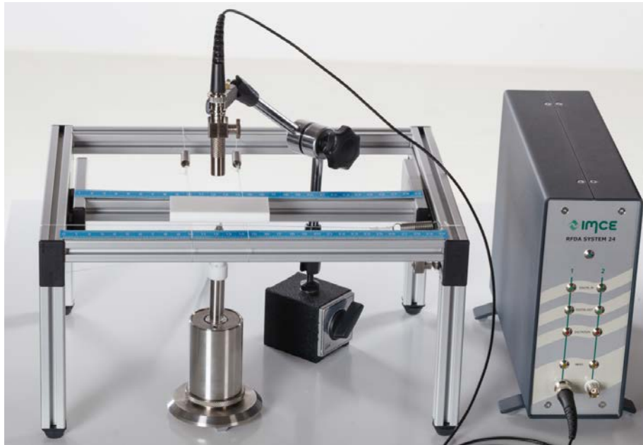
Figure 2. 9: RFDA System 24 hardware used for IE testing [64]
