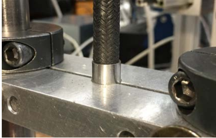
Figure 2.8: Image of adapter supporting test sample during internal pressure test
