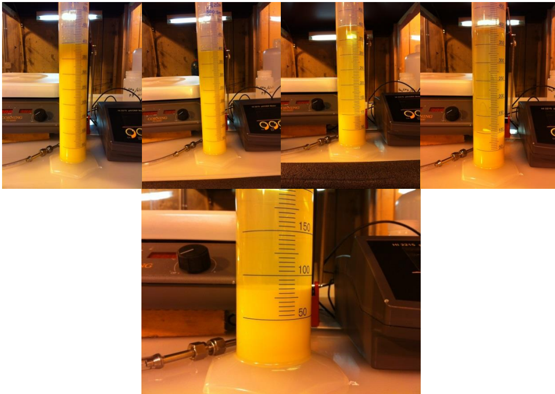
Figure 4.12 – Second Test Series, SDU settling after 2 hour digestion
