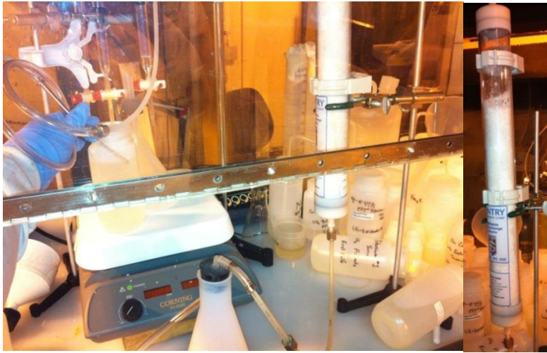
Figure 4.49 – Calcite column apparatus.
