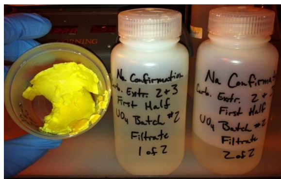
Figure 4.46 – Fifth Test Series, Batch 2, UO 4 filter cake (left) and filtrate (right).
