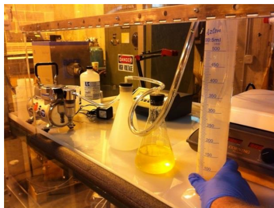
Figure 3.3 – Vacuum apparatus system
