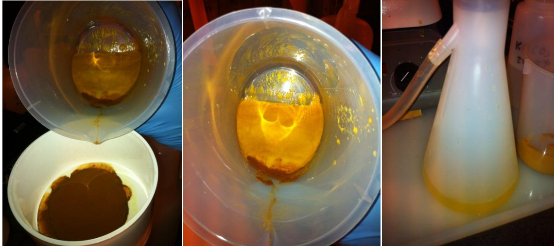
Figure 4.33 – Third Test Series, Third Carbonate Extraction filtration. Dark brown solids on filter are mostly iron; the yellow solids indicate the presence of even more uranium. It was determined that the potassium series made total uranium extraction too difficult. The yellow liquid on the left is the third carbonate extraction filtrate.
