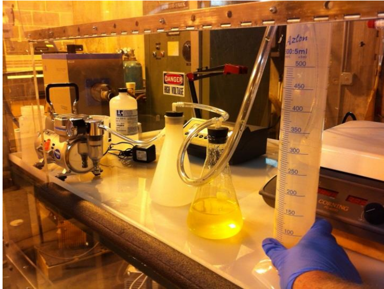
Figure 4.6 – Siphoning off supernate liquid before filtering out \text{Fe}(\text{OH})_3 solids
