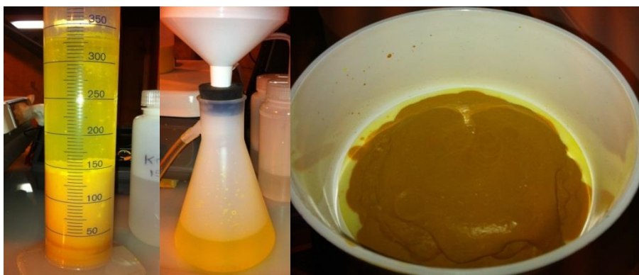
Figure 4.29 – Third Test Series, First Carbonate Extraction. High volume of solids on filter led to the belief that not all of the uranium had been extracted, so a second attempt was made.
