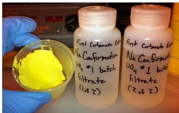
Figure 4.44 – Fifth Test Series, Batch 1, \text{UO}_4 filter cake (left) and filtrate (right).
