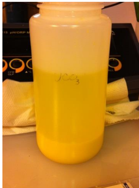
Figure 4.15 – Uranyl Carbonate Solution after overnight settling. Yellow sediment at the bottom shows that not all of the SDU has been converted.
