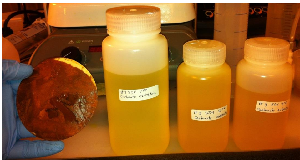
Figure 4.40 – Fifth Test Series SDU Carbonate Extraction 3. The final bit of deep brown residue is on the left and all three carbonate extractions are on the right.
