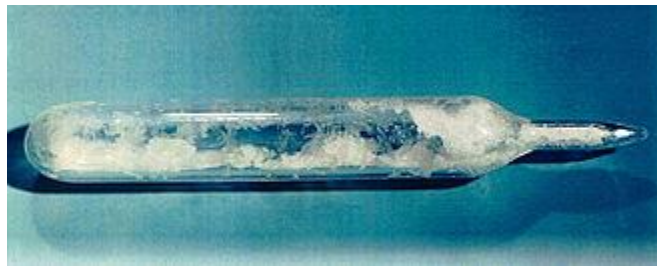
Figure 1.2 – UF 6 crystals in a small glass ampoule (4)
