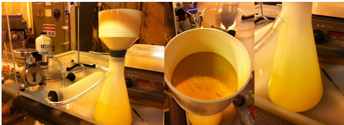
Figure 4.13 – Filtration set-up, SDU Filter Cake, SDU filtrate (NaF Solution)
