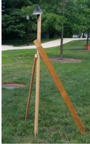
(a) Corner reflector, RCS = 1.94m^2 .
