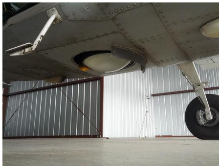
(b) Transmit and receive antennas.
