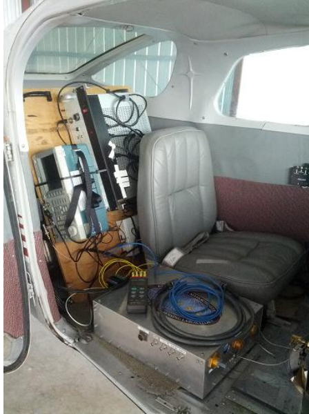
(a) Scatterometer, signal generator, ADC and power supply.
