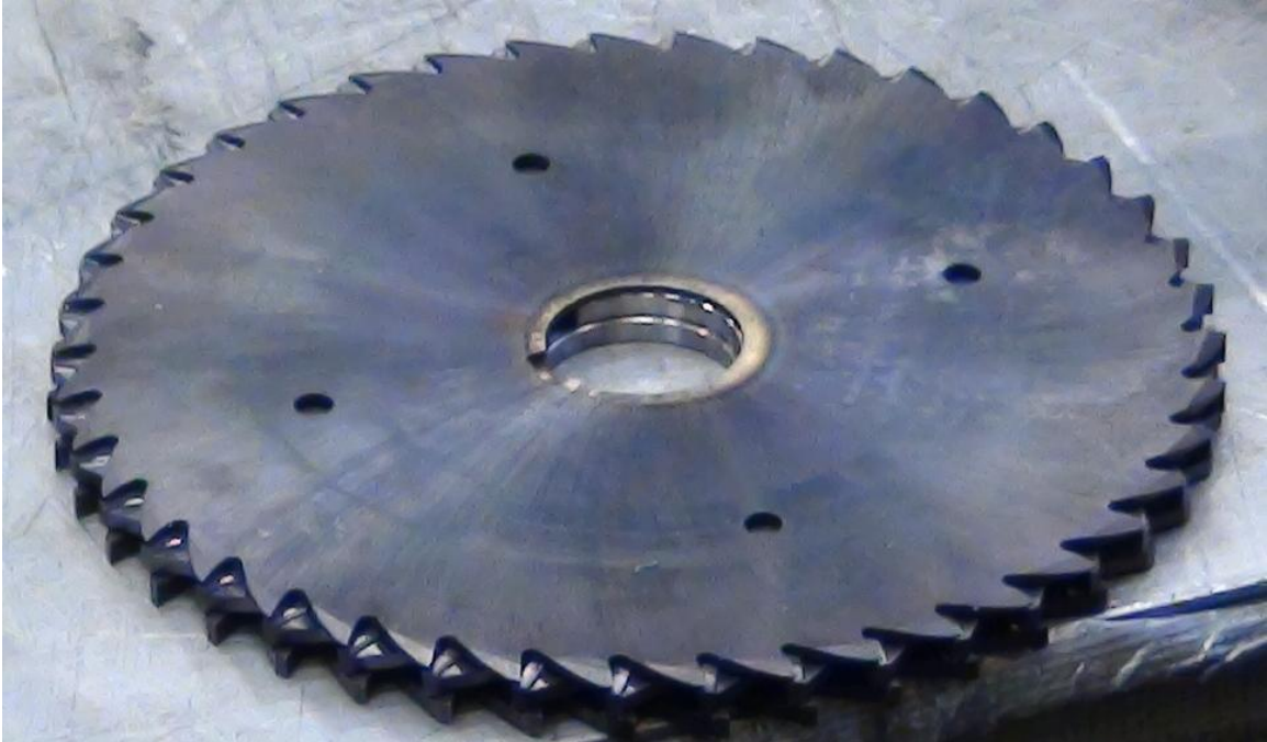
Figure 3.7. Blades used in machining the internal SC.
