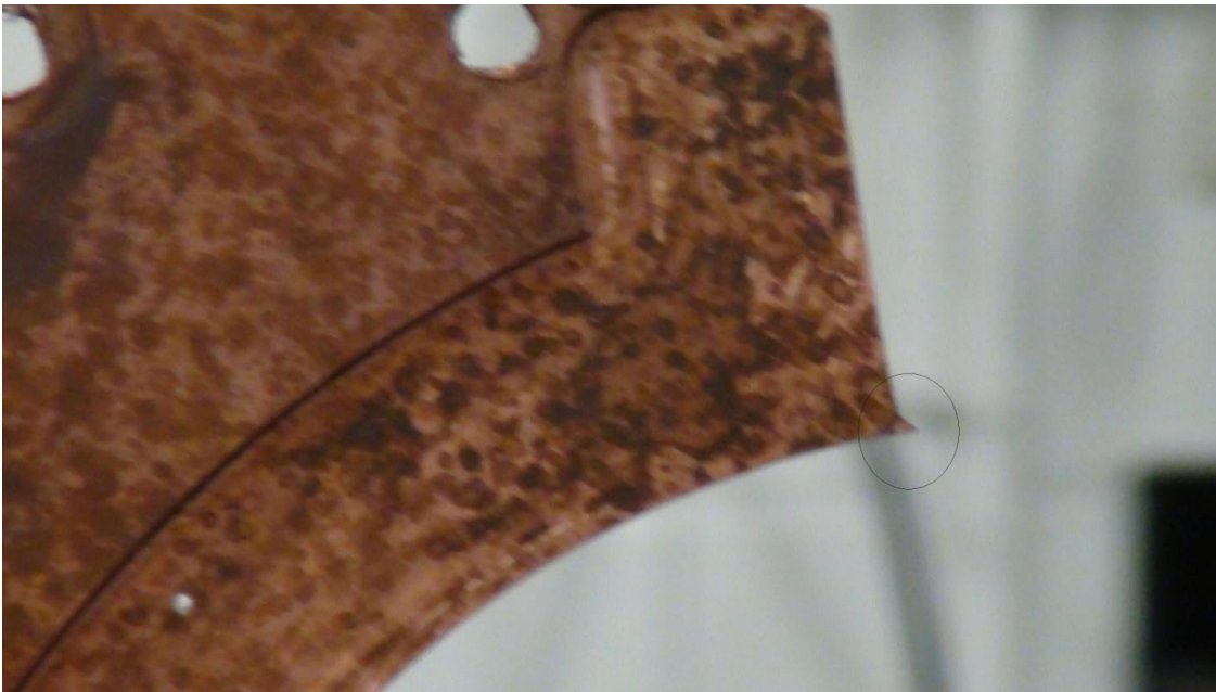
Figure 3.9. Picture of electrode used in EDM process with electrode design feature used to reduce taper circled.
