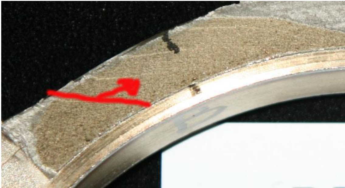
Figure 3.13. Image of DMW1 illustrating crack growth direction.
