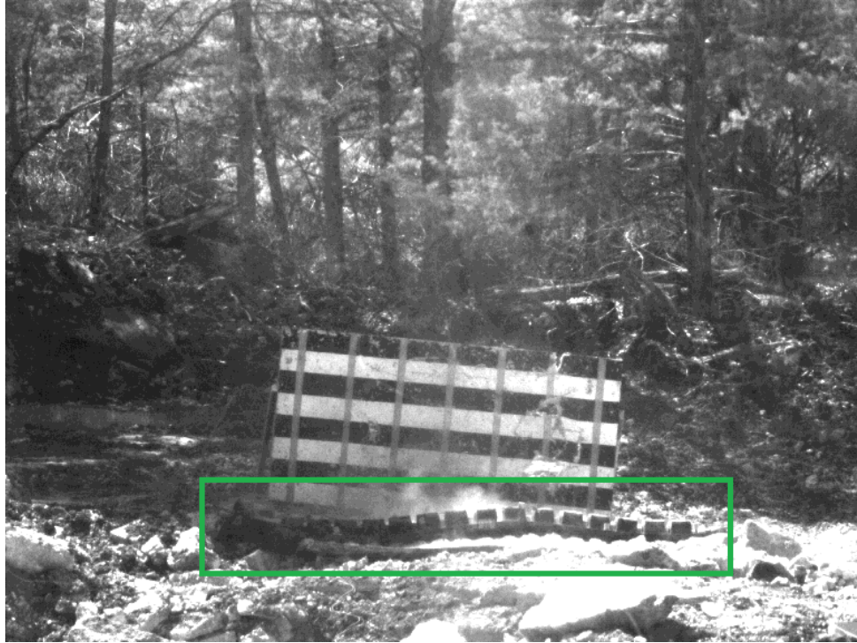
Figure 6.1 Blasting Mat Centered Over Borehole
