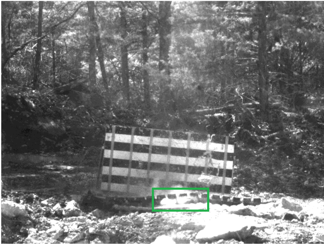
Figure 6.2 Gasses Beginning to Exit Blasting Mat During Test 3
