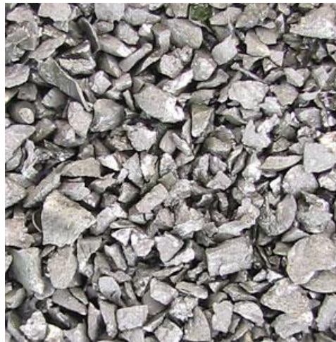
Figure 4.5 2-mm steel grit
