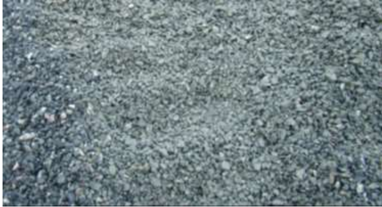
Figure 3.1. Typical Angular \frac{3}{4} " Stemming Material
