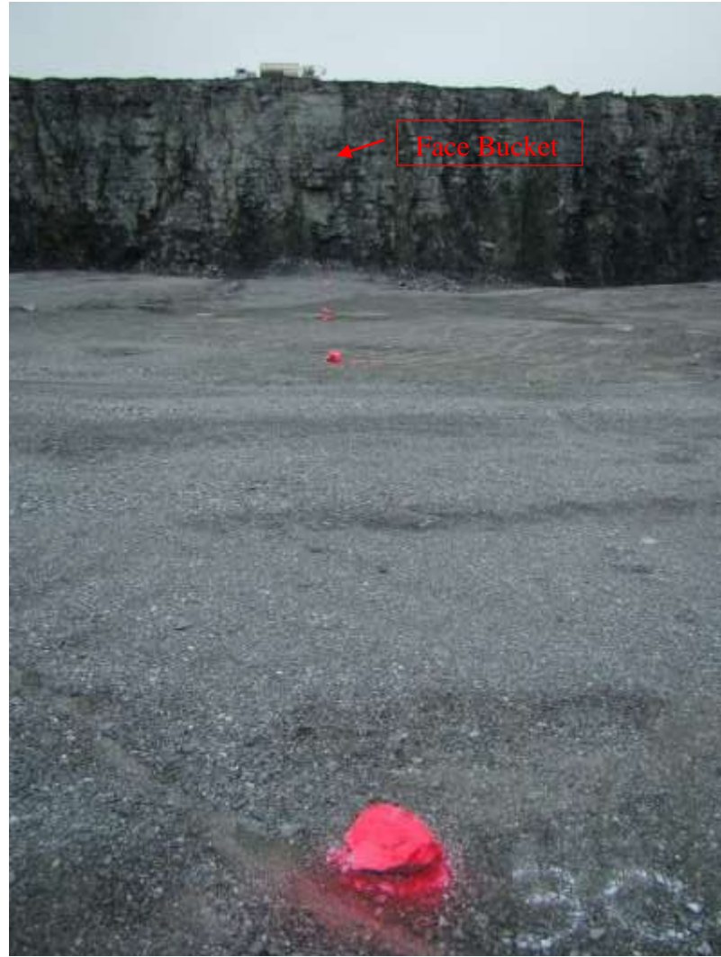
Figure 3.6. Measurement Rocks and Face Bucket
