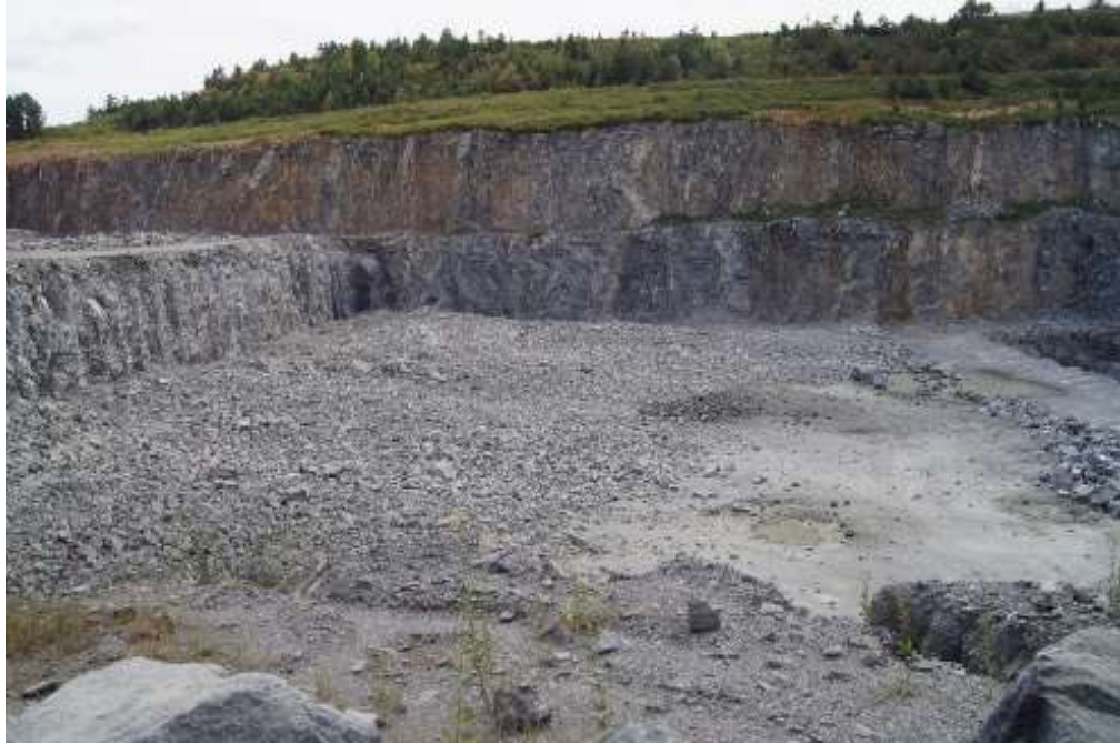
Figure 4.11. Increased Throw from 0 ms Delay (far 1/3 of photograph)
