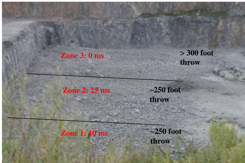
Figure 4.10. Increased Throw from 0 ms Delay
