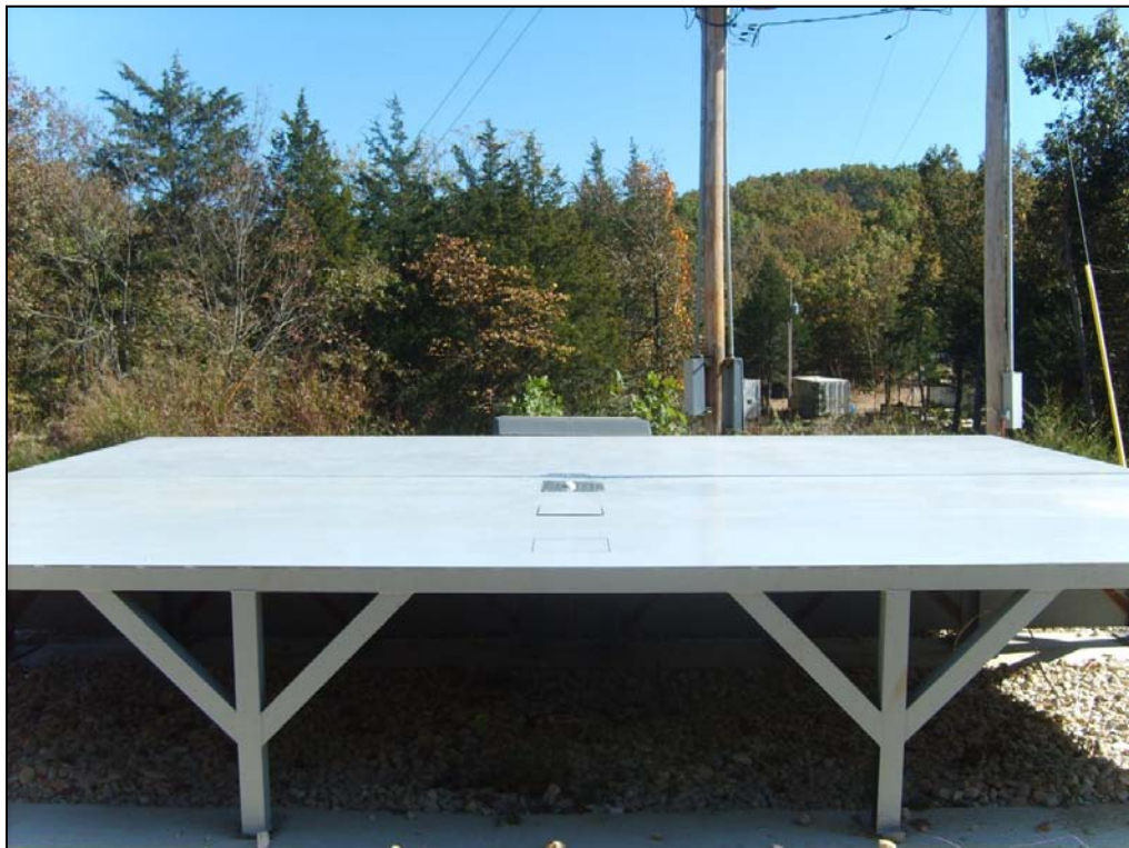
Figure 3.1. Free-field setup of the blast table with a 73 gram charge at a 387 mm standoff distance.
