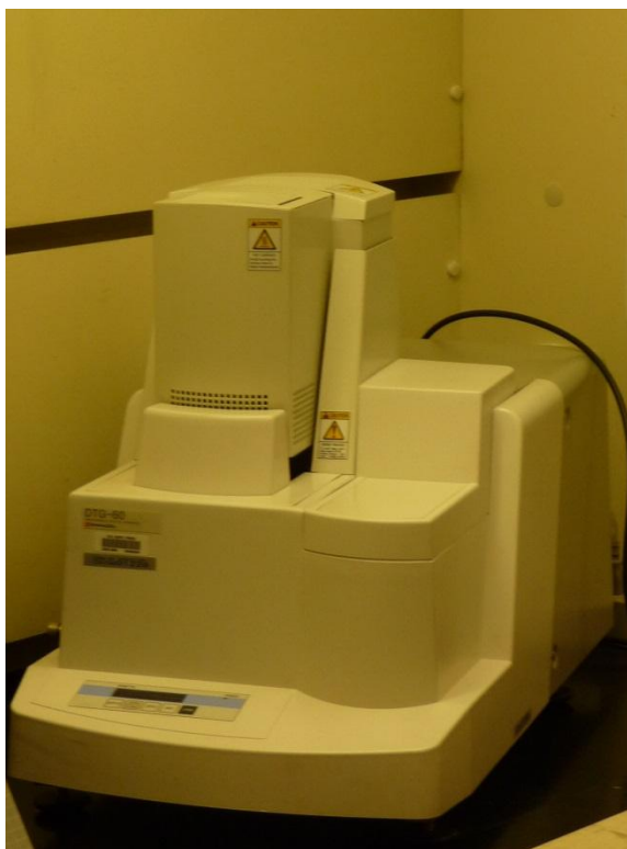
Figure 3.1. Installation of DTG-60
