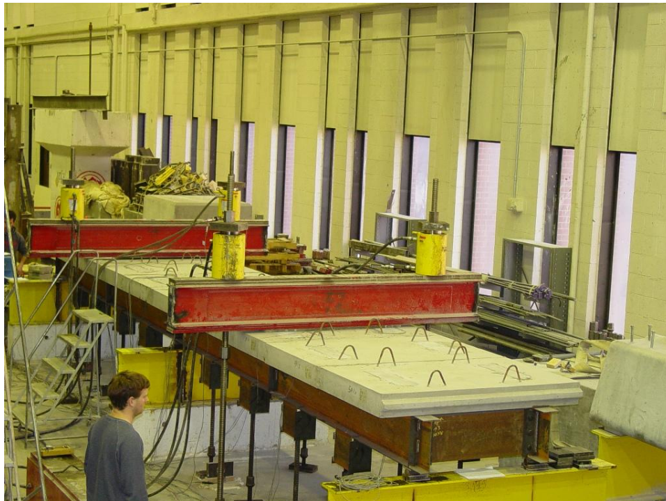
Figure 3-36. Ultimate load test setup.
