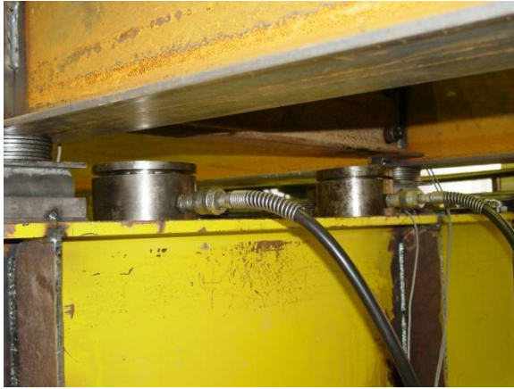
Pancake jacks used to shim the system
