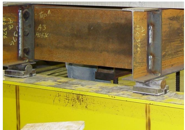
End bearings with sliding surface
