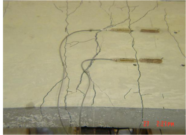
b) Crack pattern over the center support
