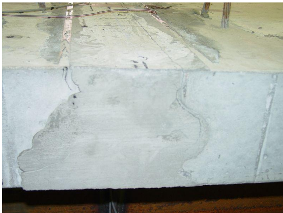
Cracking at closure region
