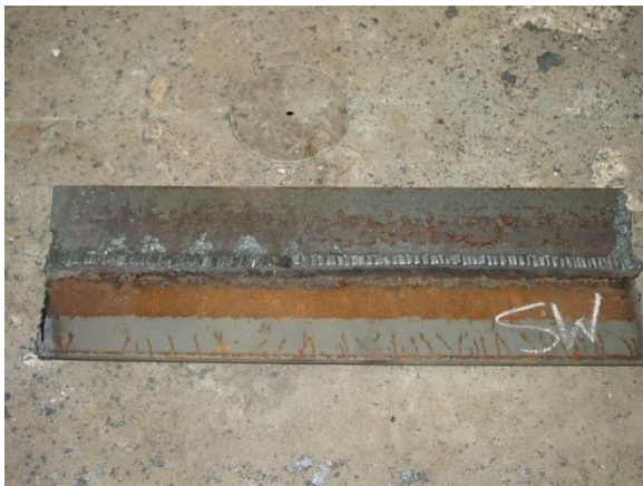
Torch cutting the bottom flange
