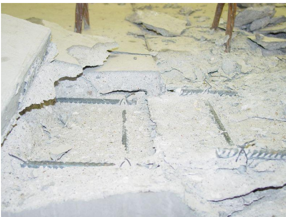
Precast panel reinforcement
