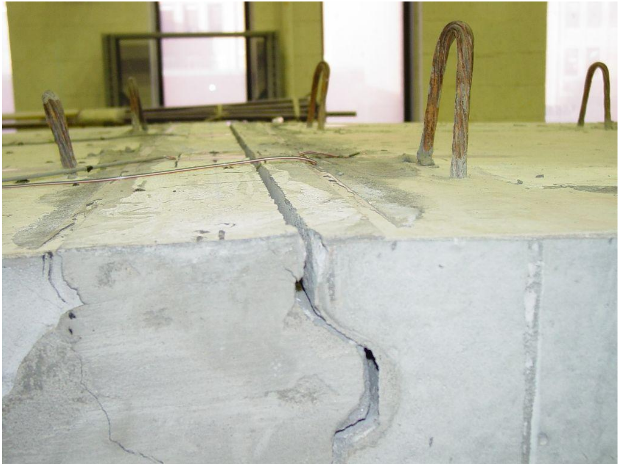
Figure 4-31. Crack at the closure region due to tensile force over interior support
