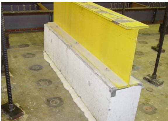
Supporting beam leveled with hydro-stone
