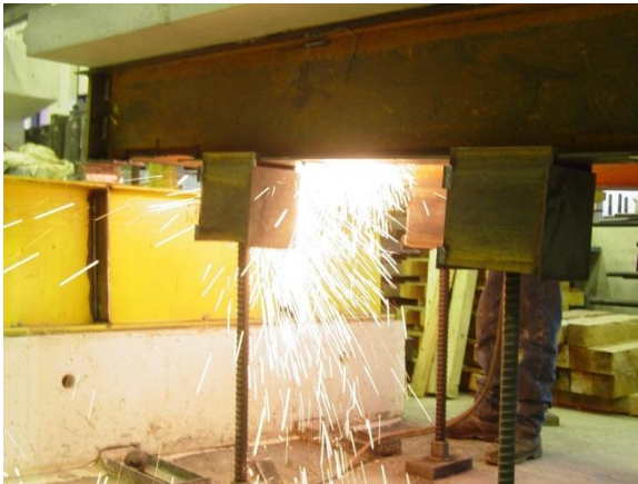
Torch cutting the bottom flange
