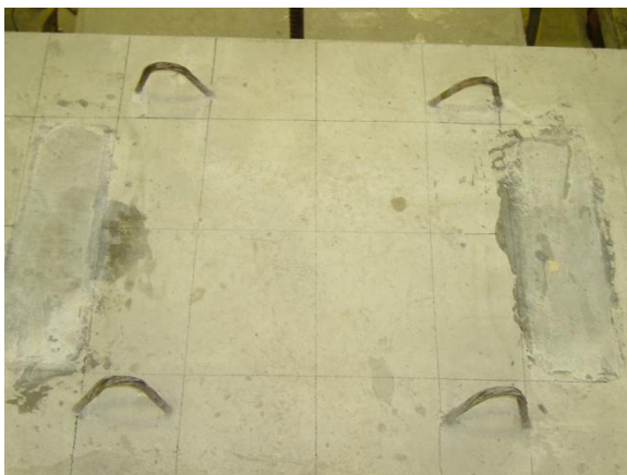
Lines drawn to guide during core removal
