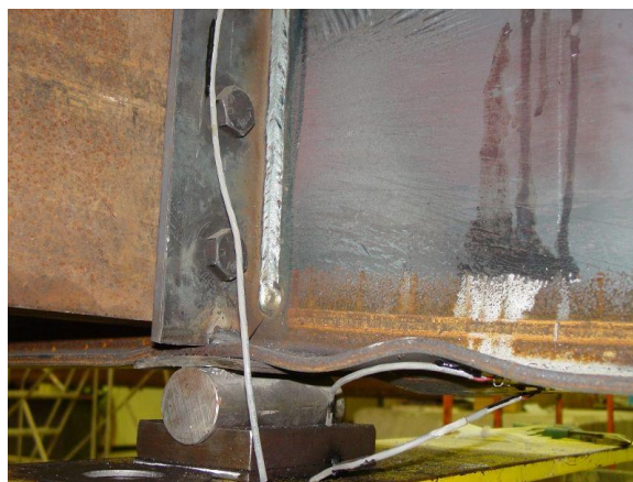
Close-up flange buckling (south girder)
