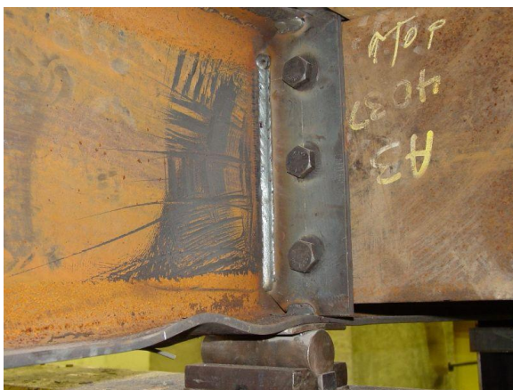
Close-up flange buckling (north girder)
