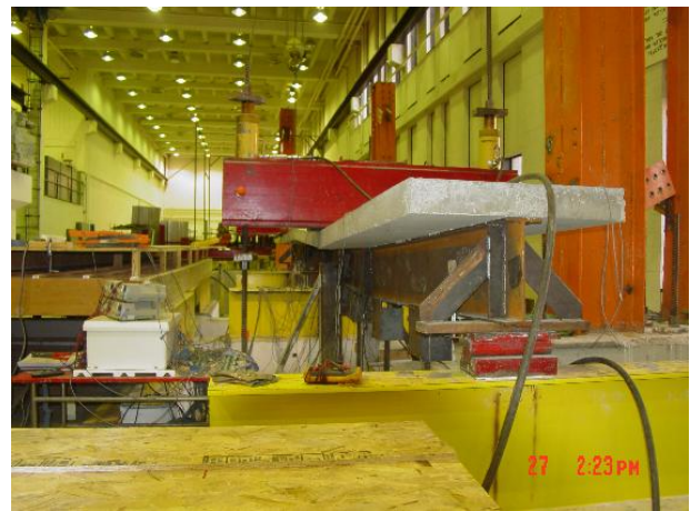
b) Large deflection (yielding/buckling) failure mode
