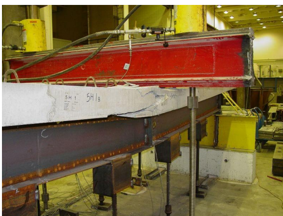
Concrete crush at west mid-span (south)
