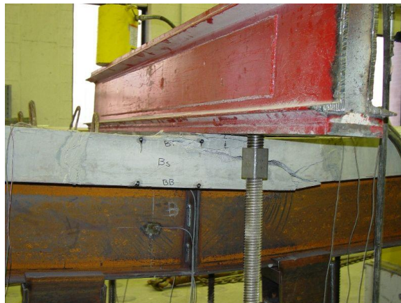
Concrete crush at west mid-span (north)
