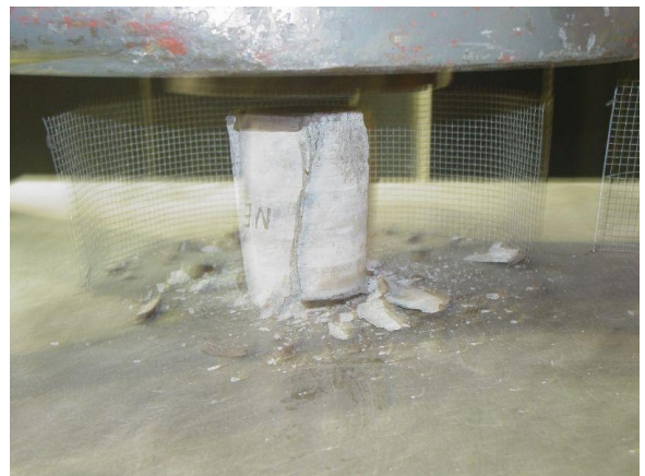
Core after tested
