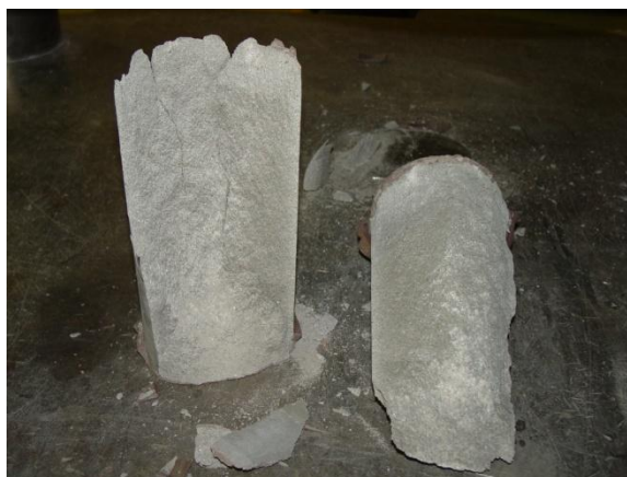
Grout cylinder after compression test
