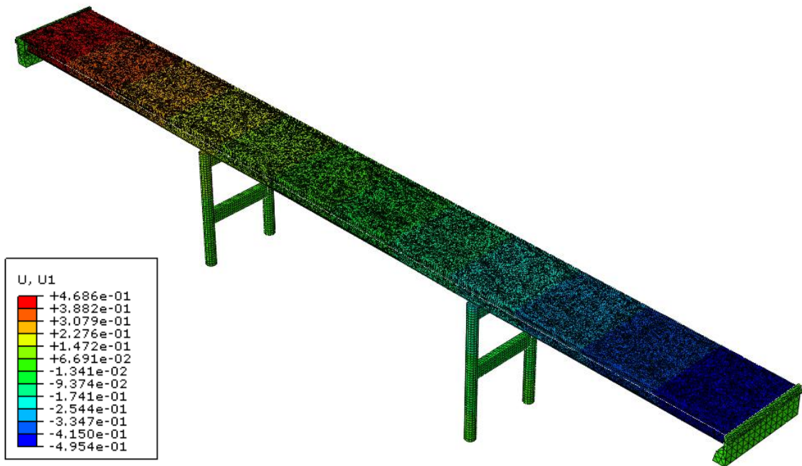
Figure 4.8: Story - Deformation Contour Plot for Temperature Loading
