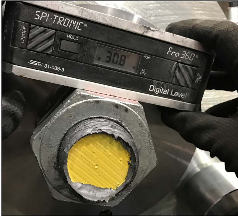
Figure 2.6 - Digital Level Measurement after Tightening
