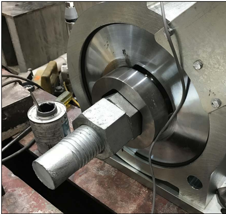
Figure 2.7 - Double Nut to Prevent Bolt Rotation
