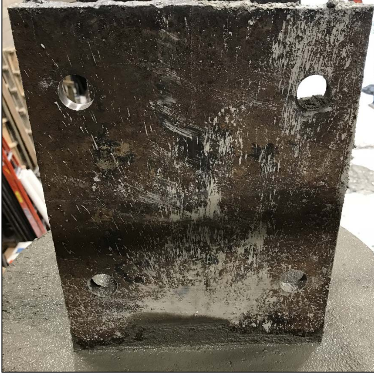
Figure 3.34 - HP10x57 Curing in Concrete
