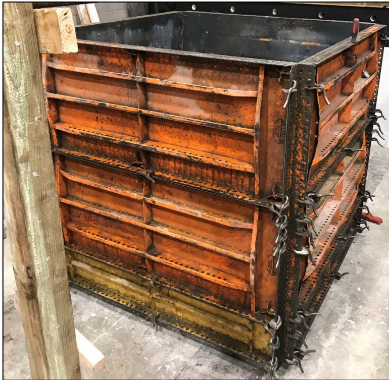
Figure 3.25 - Concrete Block Formwork
