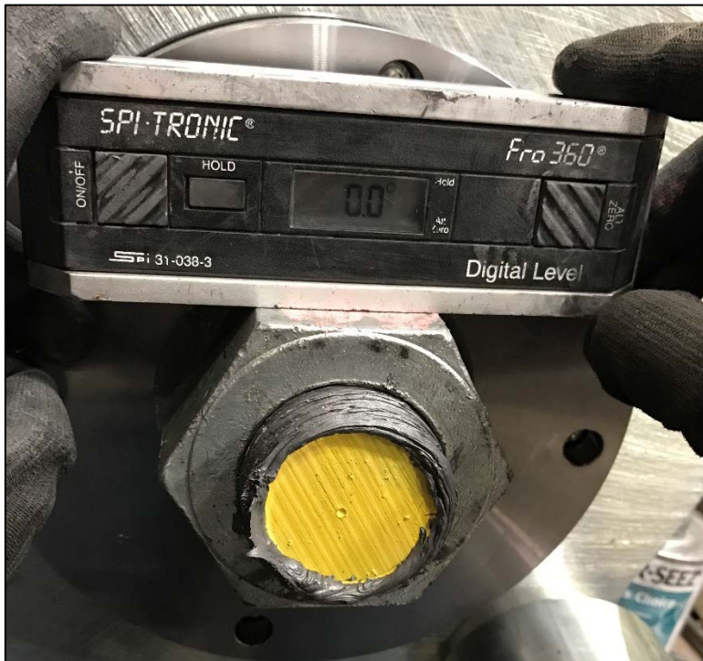
Figure 2.5 - Zeroing of Digital Level
