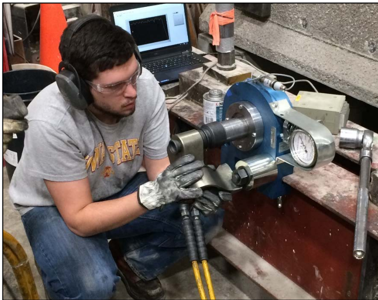
Figure 2.1 - Hydraulic Wrench Tightening
