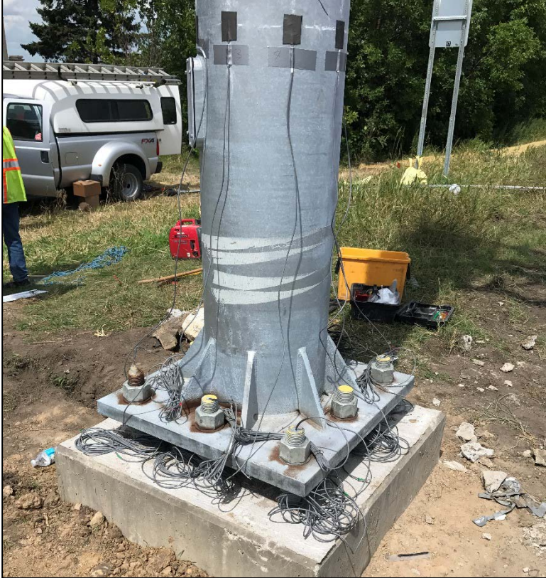
Figure 3.8 - Anchor Bolt and Post Strain Gages
