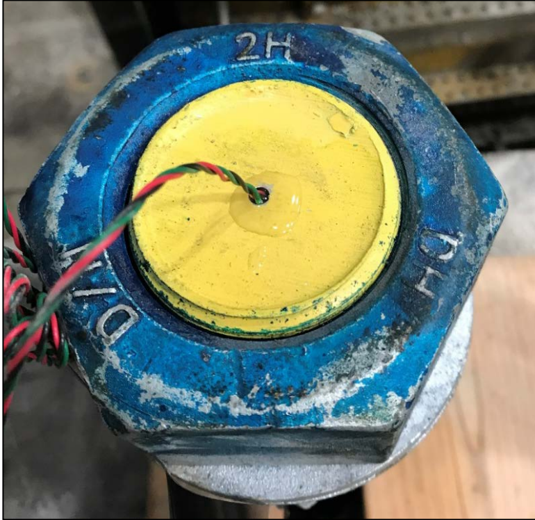
Figure 3.6 - Anchor Bolts after Strain Gage Installation
