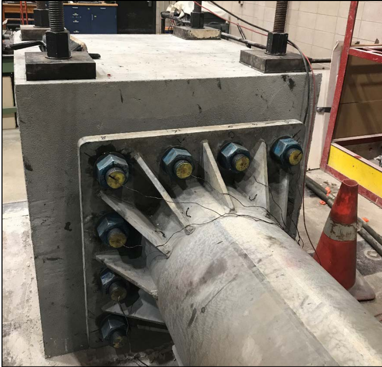
Figure 3.36 - Concrete Block Following Post-tensioning
