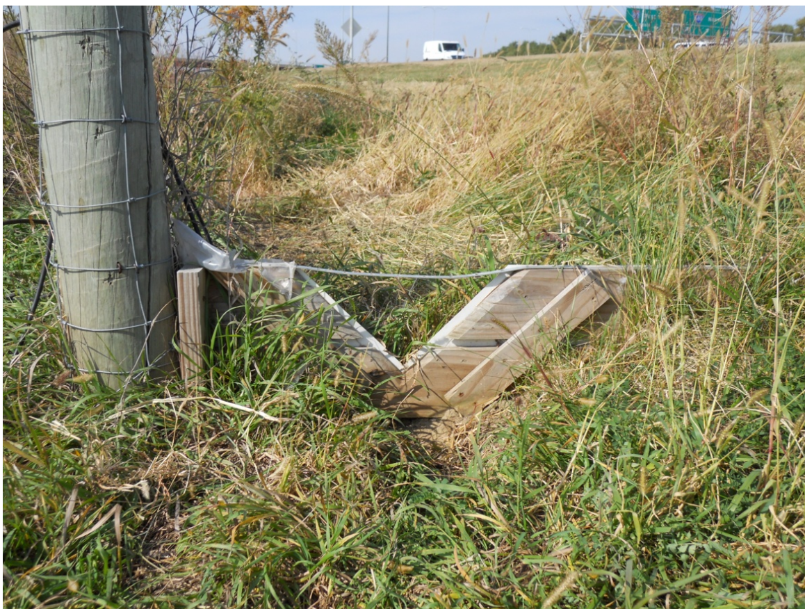
Figure 4-4: V-Notch Weir Installed at Site B
