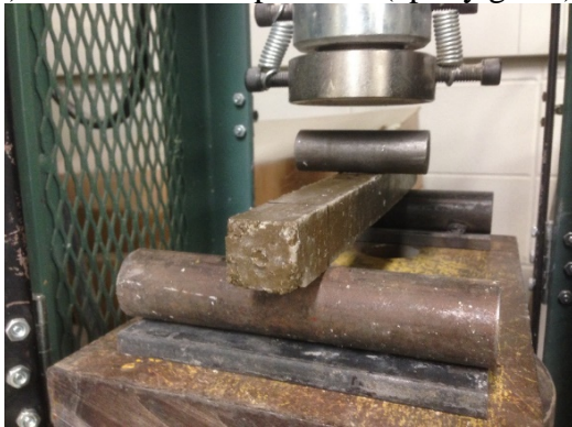
(c) Flexural tensile strength (epoxy grout)
