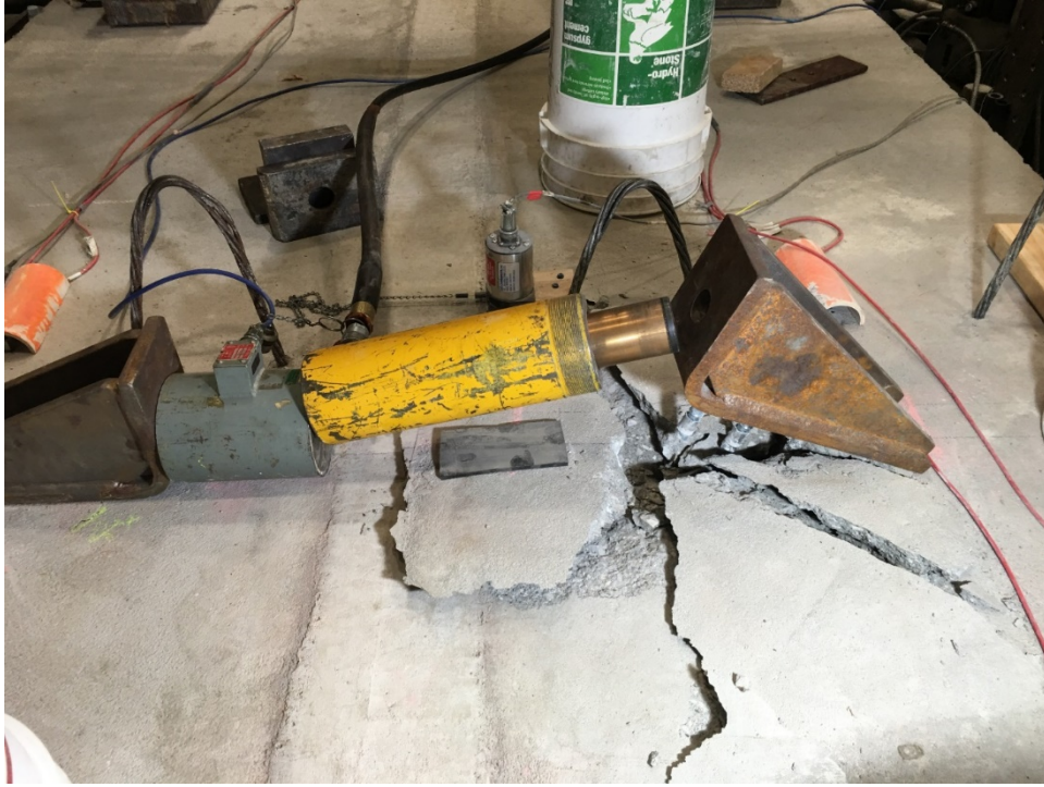
Figure 5-12 Crashed Box Girder due to Horizontal Load
