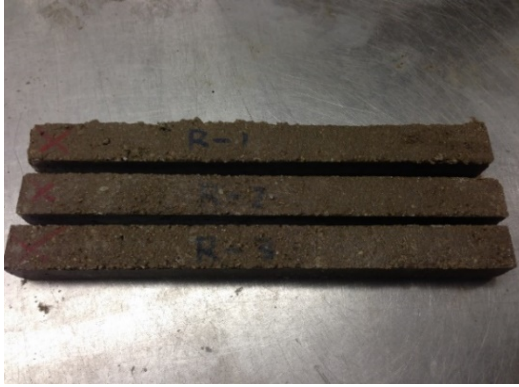
(a) 1"×1"×11.25" specimen (epoxy grout)
