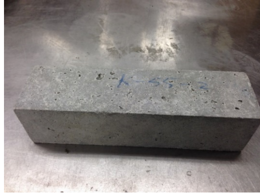
(b) 3"×3"×11.25" specimen (concrete)
