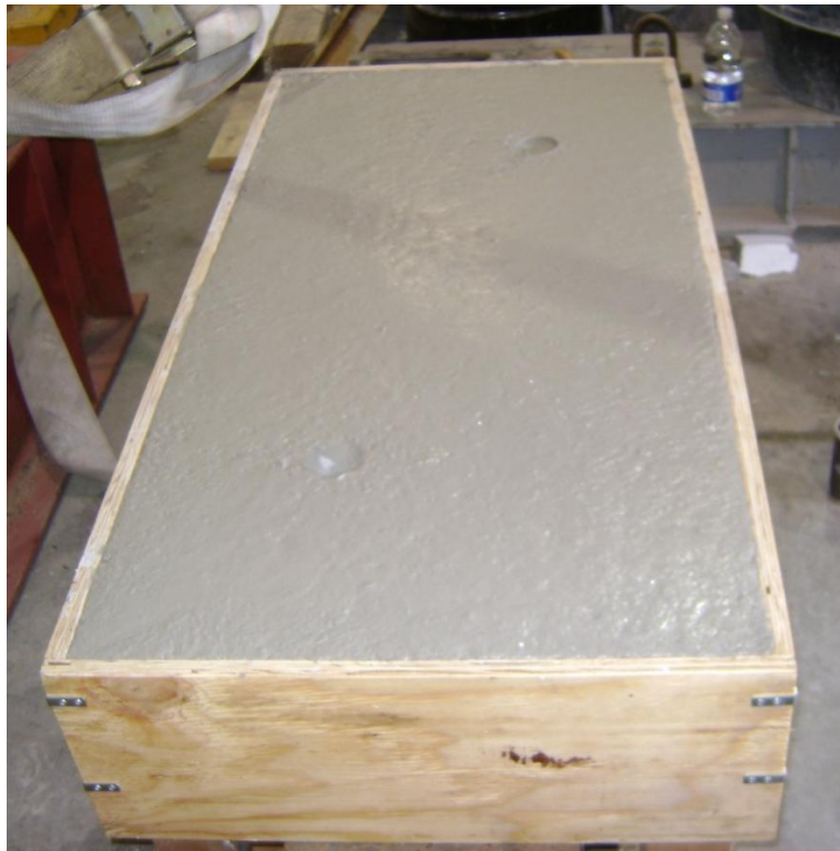
Figure 27: Specimen after Concrete Placement
