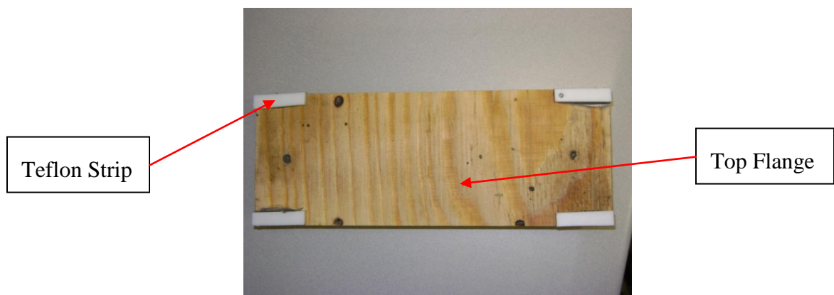
Figure 17: Top Flange with Bearing Strips
