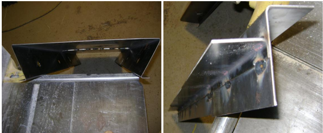
Figure 31: Fabricated Pieces before Installation
