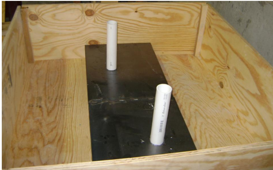
Figure 33: Specimen with Formwork
