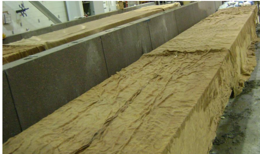
Figure 56: Specimens Covered During Initial Curing
