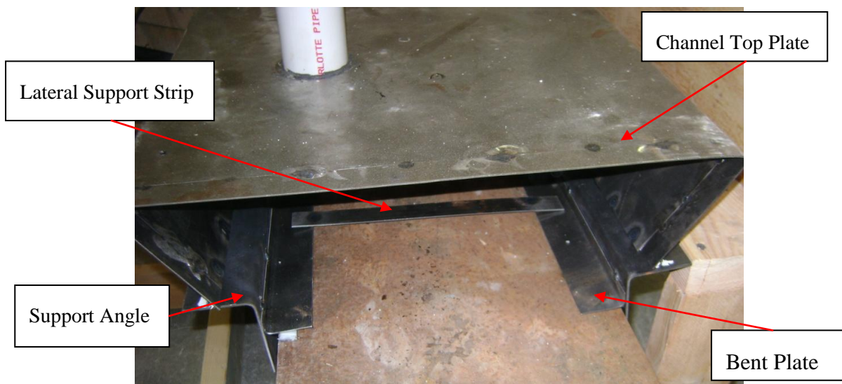
Figure 22: View of Cross Section
