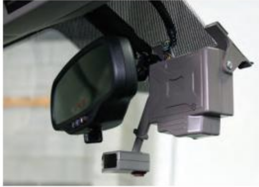
Figure 8. Interval Video Camera and Passive Alcohol Sensor (Campbell, 2012)
