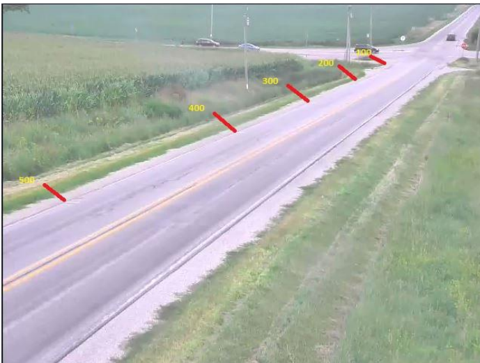
Figure 4-6: Marks placed in video frame to ensure distance are visible to data reductionists
