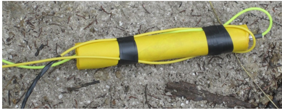
Figure 3-4: Primed Stick of Dynamite
