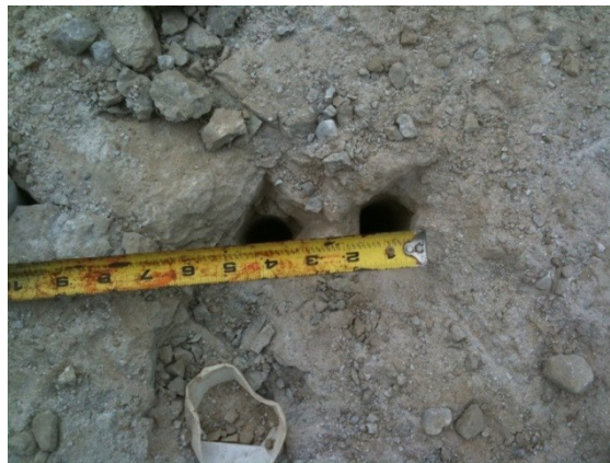
Figure 3-10: Measurement of Hole Separation on Surface
