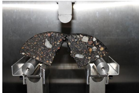
(b) an SCB specimen with fracture
