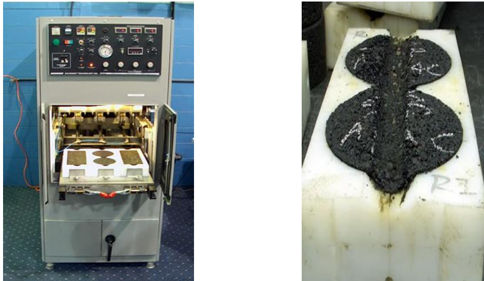
Figure 3.13 APA Test Station and Specimens after Testing
