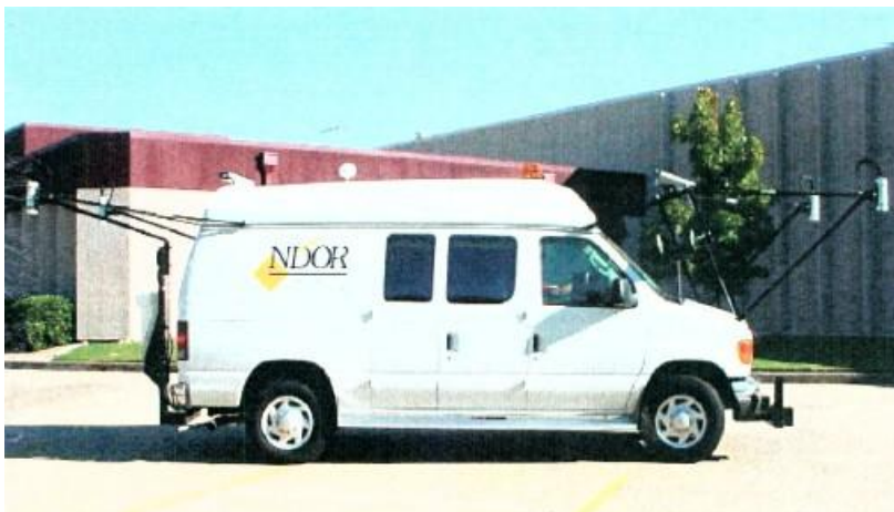
Figure 3.22 A Vehicle Used to Monitor Pavement Performance
