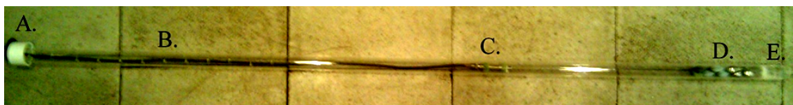
Fig. 3. Movable detector tube assembly. A. Cap detector is suspended from. B. Preset suspension locations. C. ^3\text{He} neutron detector. D. Lead weights. E. Acrylic stopper.
