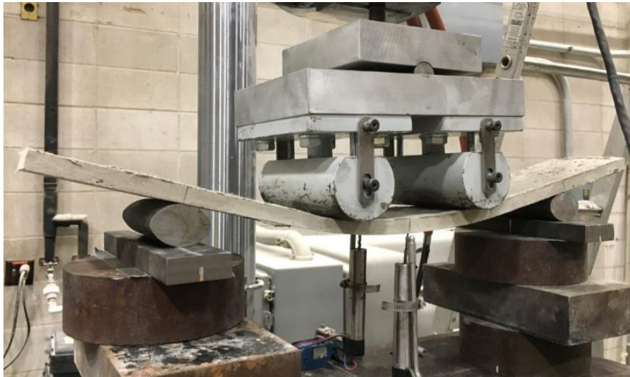
Figure 4. EGC slab under bending test
