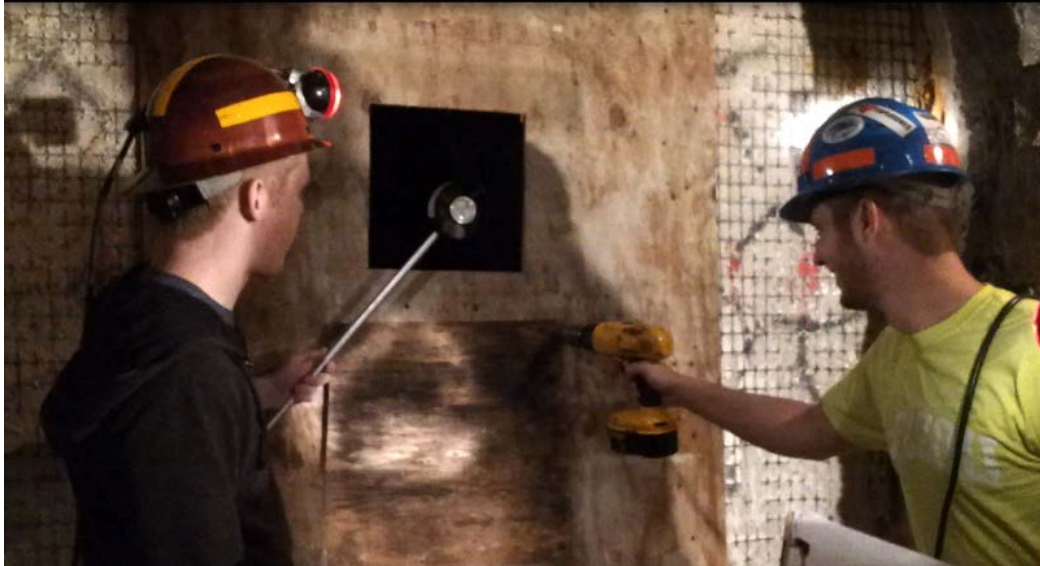
Figure 3.7. Measuring leakage at Missouri S&T Experimental Mine stopping
