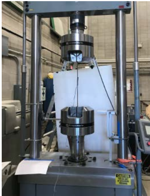
Figure 3-2. Steel Uniaxial Tensile Test Setup
