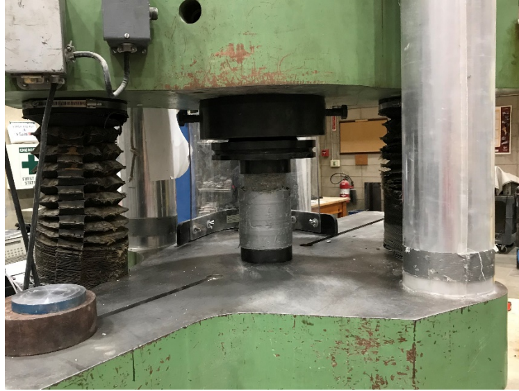
Figure 3-1. SATEC Machine for Cylinder Test
