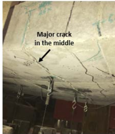
Figure 3-20. Major crack in mid-span of the wall
