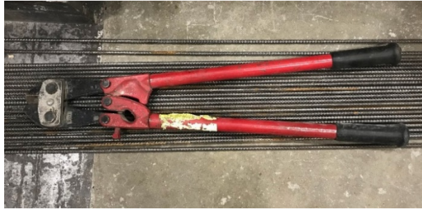
Figure 3-4. Bolt Cutter Used in Cutting NO.2 Bars
