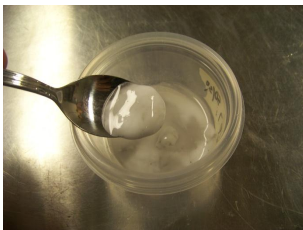
Figure 4.23: Potassium Acetate Reacted with Road Salt
