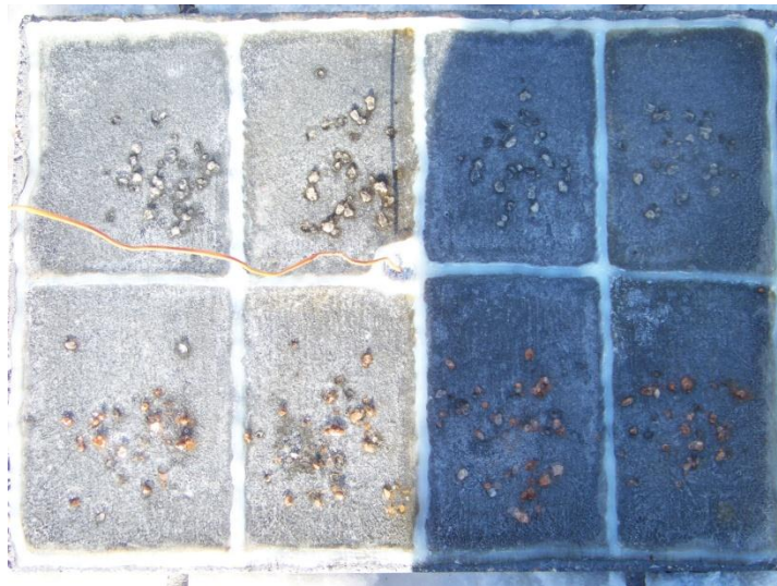
Figure 3.15: Deicing Samples in Shaded and Sunlit Areas
