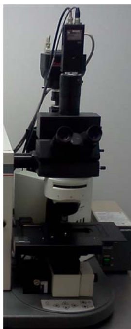
Figure 4.4 Microscope unit portion of the Laser Scanning Cytometer
