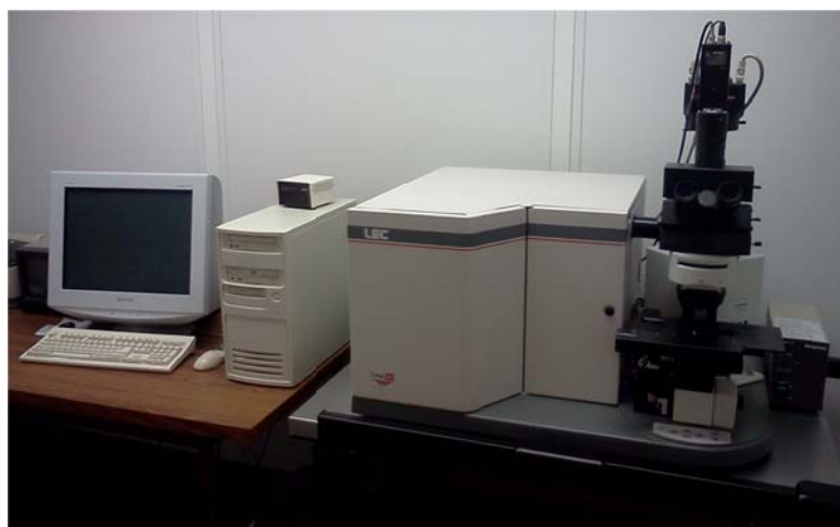
Figure 4.2 Laser Scanning Cytometer laboratory set-up
