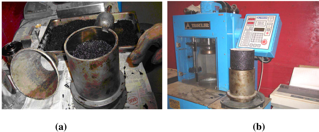
Figure 3.9 - Loose mixtures into the SGC mold and compacted HMA sample
