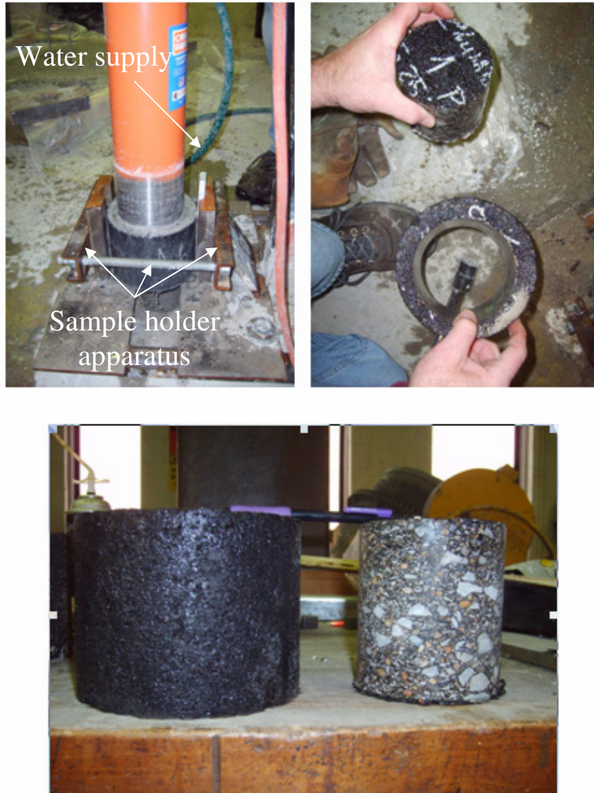
Figure 3.12 - Coring the SGC compacted HMA mixture
