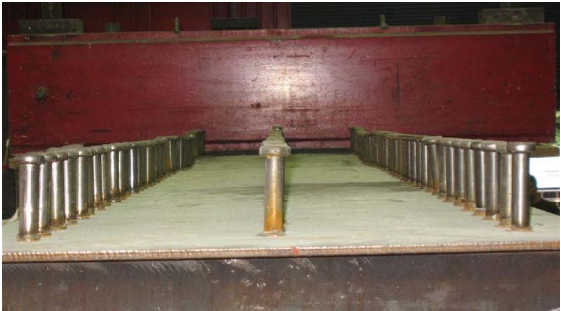
Figure 3-42 Test B1 top flange at 140kip
