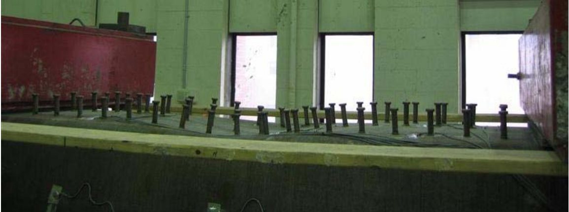
Figure 3-44 Top flange at 137 kip after failure
