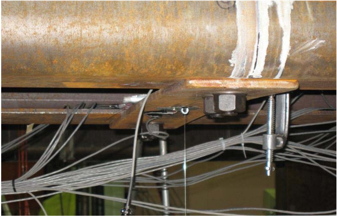
Figure 3-41 Test B1 tie plate at 140kip
