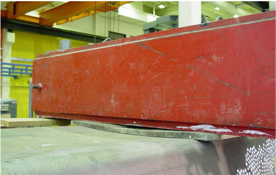
Figure 3-7 Top flange during loading
