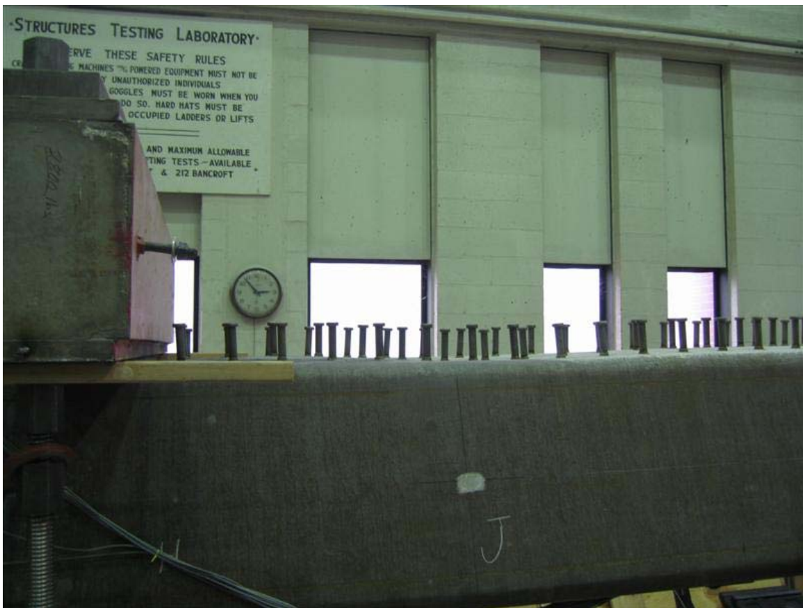
Figure 3-45 Girder outside load points at 137 kip on way back down
