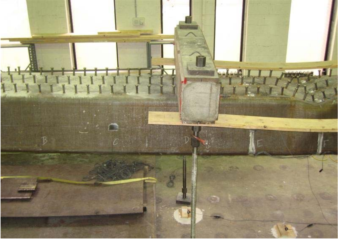
Figure 3-47 Permanent deformation after unloading
