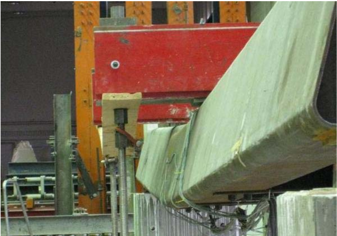
Figure 3-46 Girder deflection after unloading
