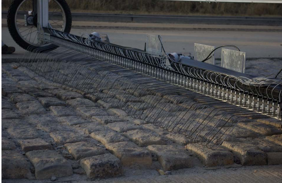
Figure 7.15: Belgian paving at Gerotek Test Facilities
