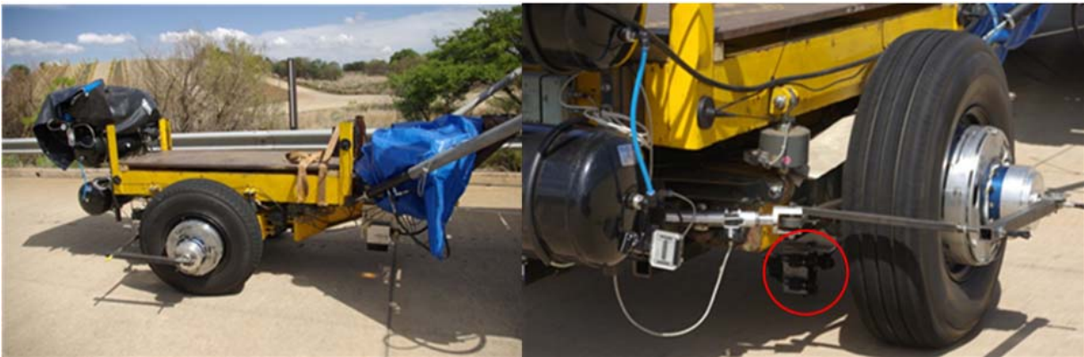
Figure 6.7: Tyre test rig, showing encircled camera mounting position
