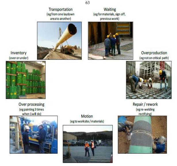
Figure (3:1) : Seven waste in construction
