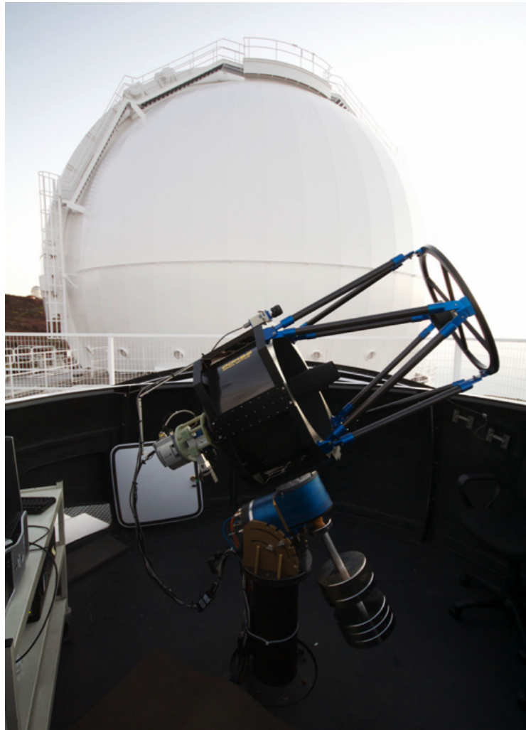
Figure 6.2: Photo of the pt5m instrument in front of the WHT dome. The telescope is a 0.5 m modified Dall-Kirkham. At the focus of the telescope the Andor iXon wavefront camera can be seen at the furthest left point, and on the inside of that the slider to move the fast photometry camera in place. To the left of the image just in frame are the Linux PC's used for data acquisition and reduction, and telescope control. (Photo credit; Vik Dhillon (University of Sheffield))
