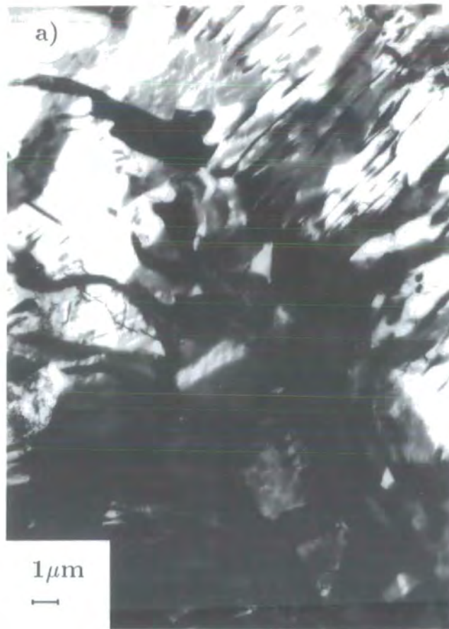
Figure 5.34 Foucault electron micrograph of undeformed 7092.
