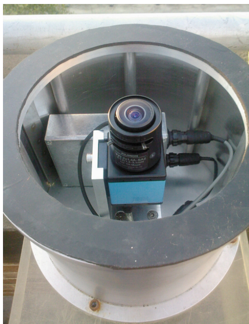
Fig. 2.5 The pictures of the Durham all-sky camera. In (a), it shows the components inside the case. In (b) shows what the camera looks like after construction.
