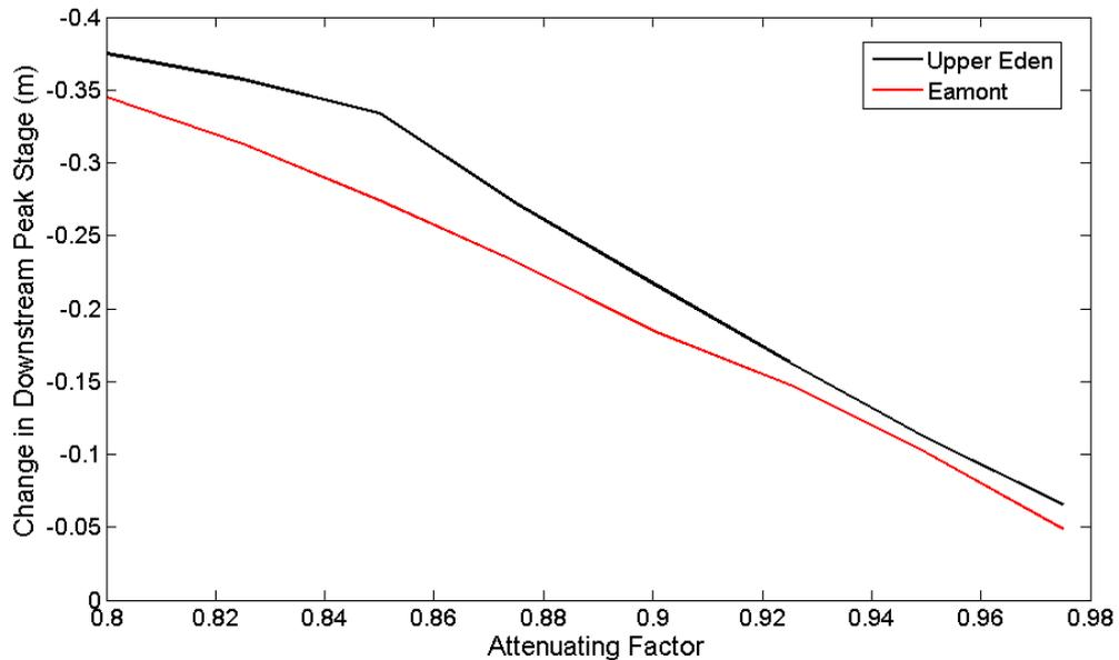
**Figure 6.33** Impact of varying degrees of attenuation of peak stage at Sheepmount.
