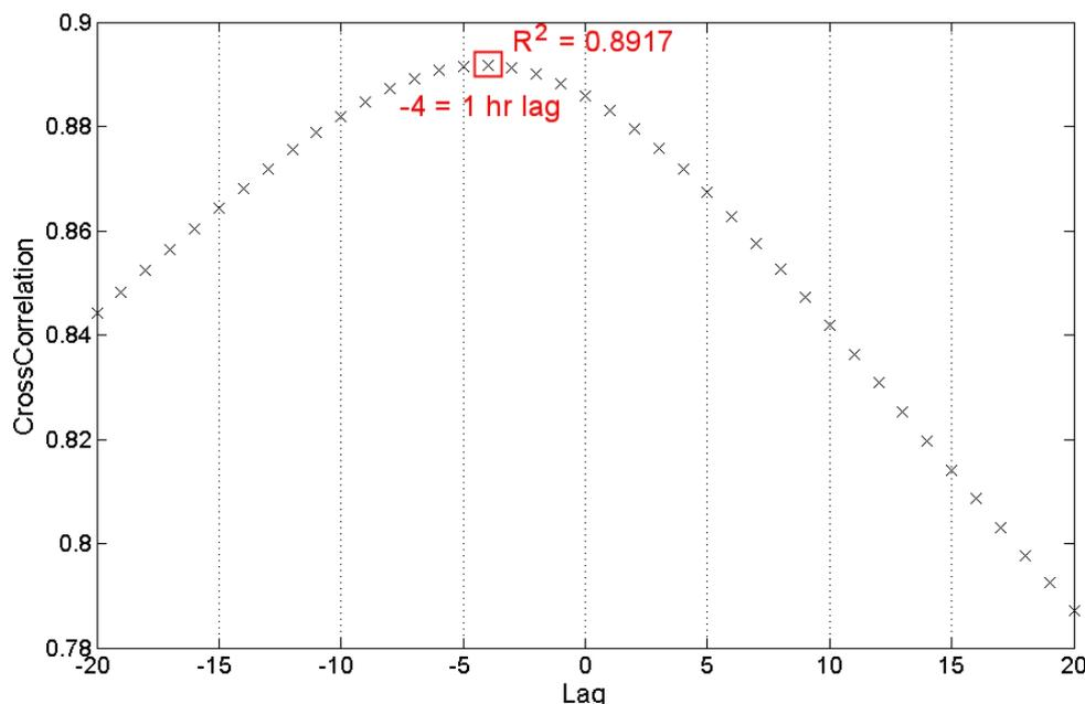
**Figure 3.24** Cross correlation plot between Eamont Bridge and Udford gauging stations. Lag refers to the data point number, which have a time step of 15 minutes. Therefore when lag = -4 = -4 \* 15 = -1 hour.
