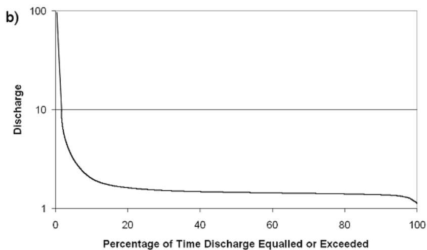
Figure 3.31b Flow Duration Curve – Discharge transformed by logarithm
