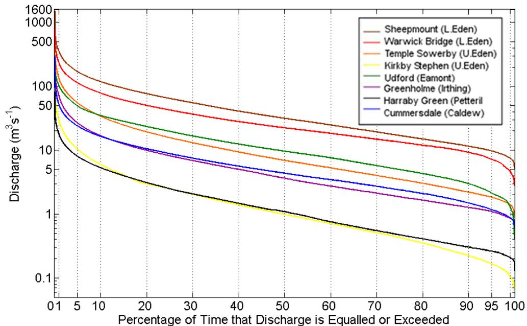
**Figure 4.2.** Flow Duration Curves for different gauging stations in the Eden catchment from 1981 to 2007
