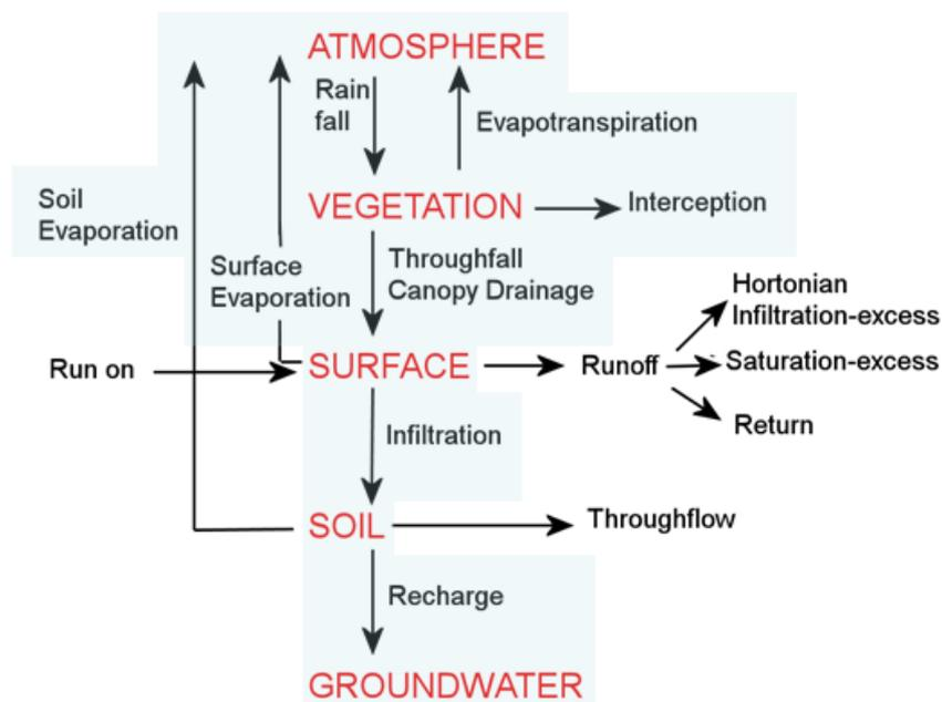
**Figure 8.2** Conceptual framework of the hydrological processes for the CRUM in individual cells (1D hydrological module cell shaded)
