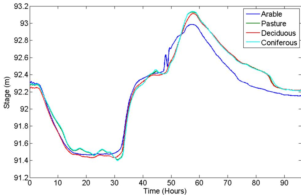
**Figure 9.43** Effect of land cover type on peak stage at the sub-catchment scale (Eamont at Udford)
