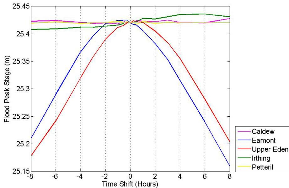
**Figure 6.28** Sensitivity of peak stage at Great Corby to timing shifts of the contributing sub-catchments hydrograph
