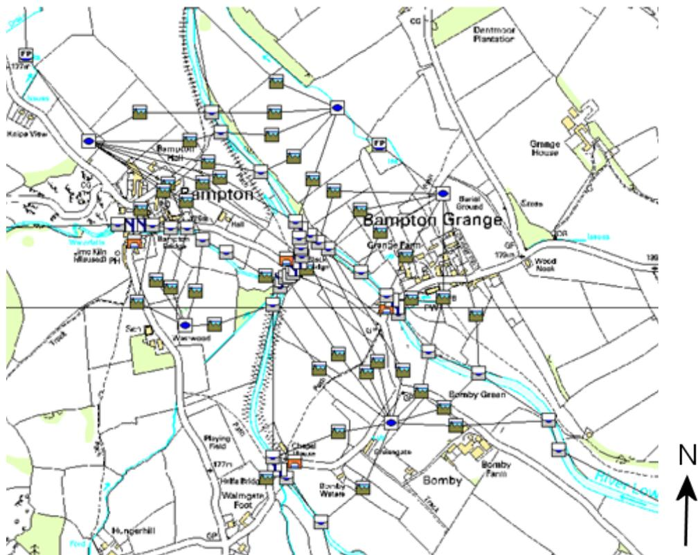
**Figure 9.23** Schematic of the Lowther iSIS model structure at Bampton showing floodplain representation through reservoir units
