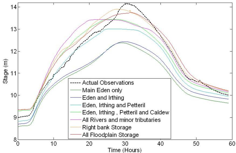
**Figure 5.3** Hydrograph for January 2005 flood at Sheepmount compared to model simulations
