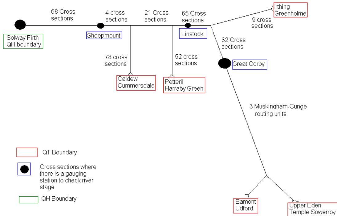
**Figure 5.2** Schematic of Full Eden model structure
