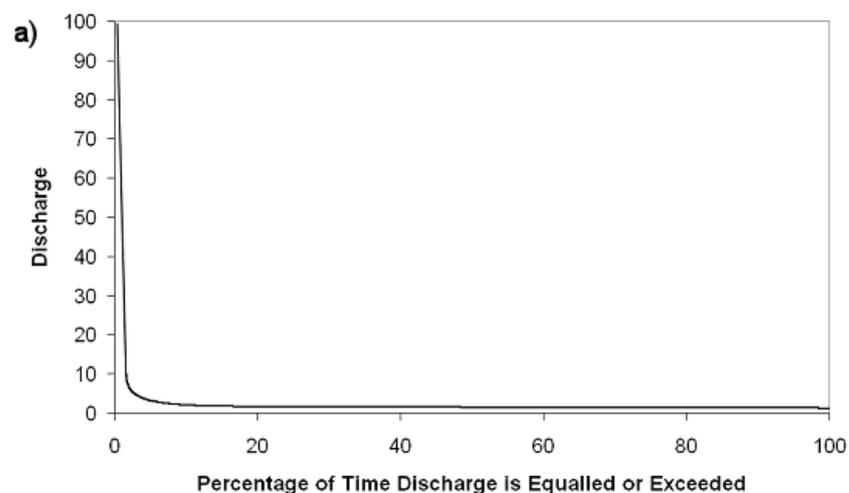
Figure 3.31a Flow Duration Curve – untransformed axes
