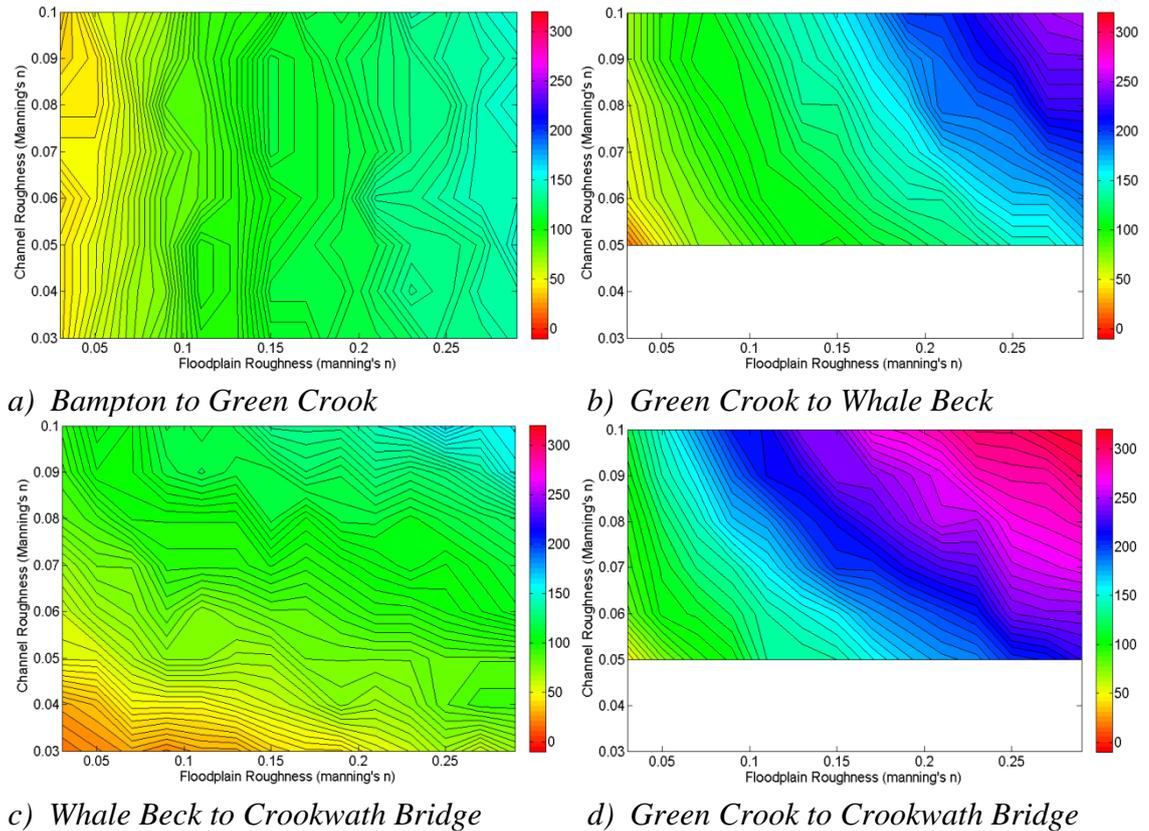
**Figure 9.37** Impact of roughness modification on sub-catchment scale (Askham) peak flow timing for the 10<sup>th</sup> January 2005 flood event.
