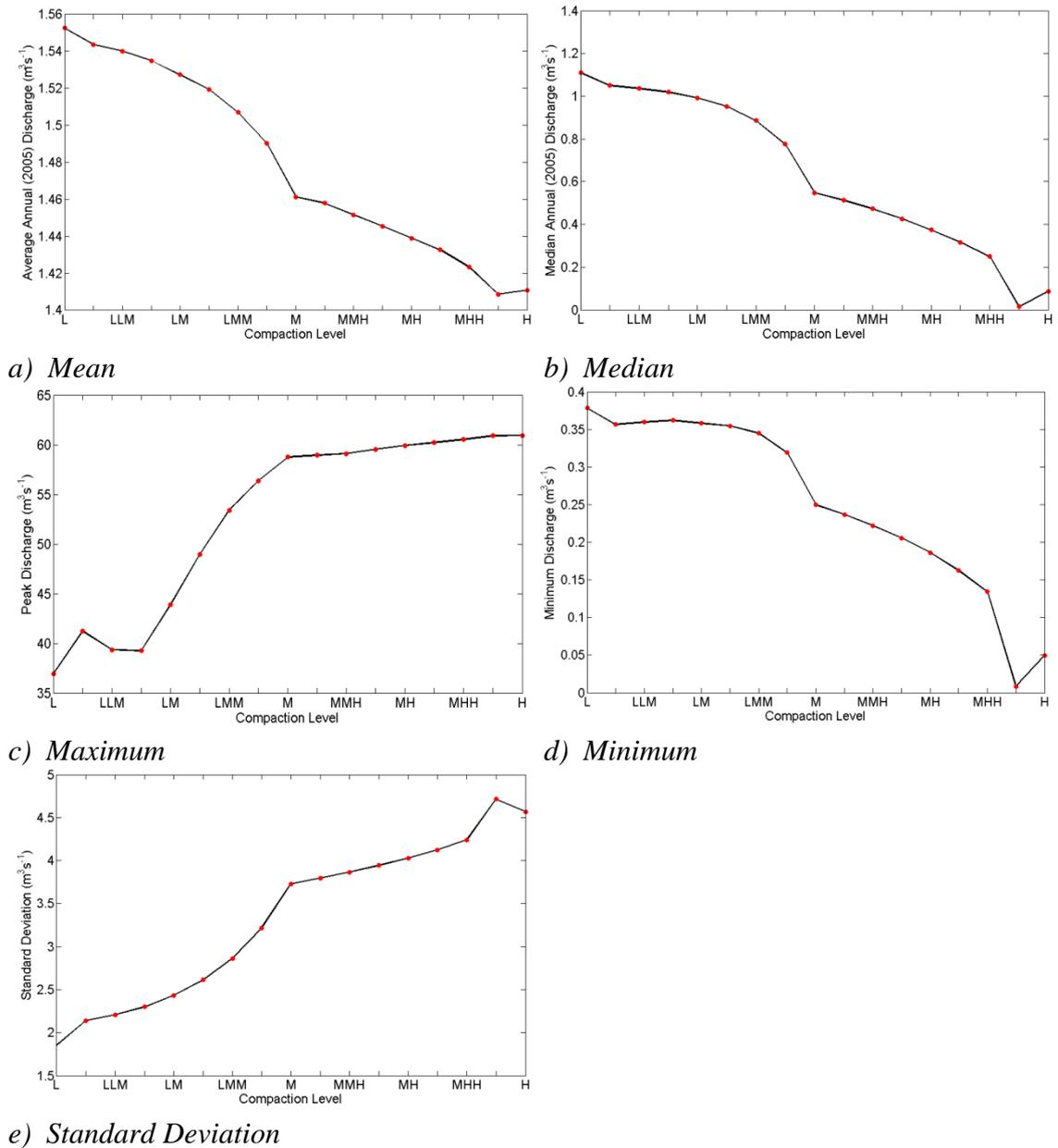
**Figure 9.8** Descriptive statistics for discharge simulated by continuum of compaction scenarios (where L = Light, M = Moderate, and H = Heavy compaction, and the rest are linearly interpolated e.g. LLM = Light Light Moderate)
