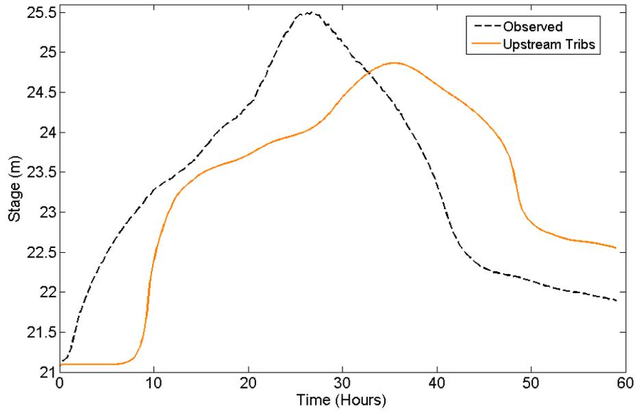
**Figure 5.5** Simulated and Observed Hydrograph at Great Corby
