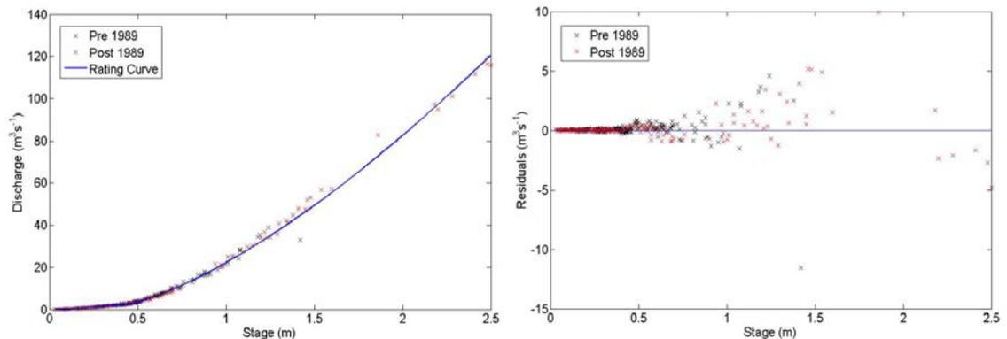
a) Rating curve and spot gaugings      b) Residuals of spot gauging from curve
