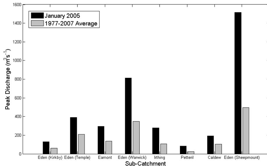
**Figure 6.8** Comparison of the January 2005 flood with the long term average in terms of peak magnitudes from each sub-catchment.
