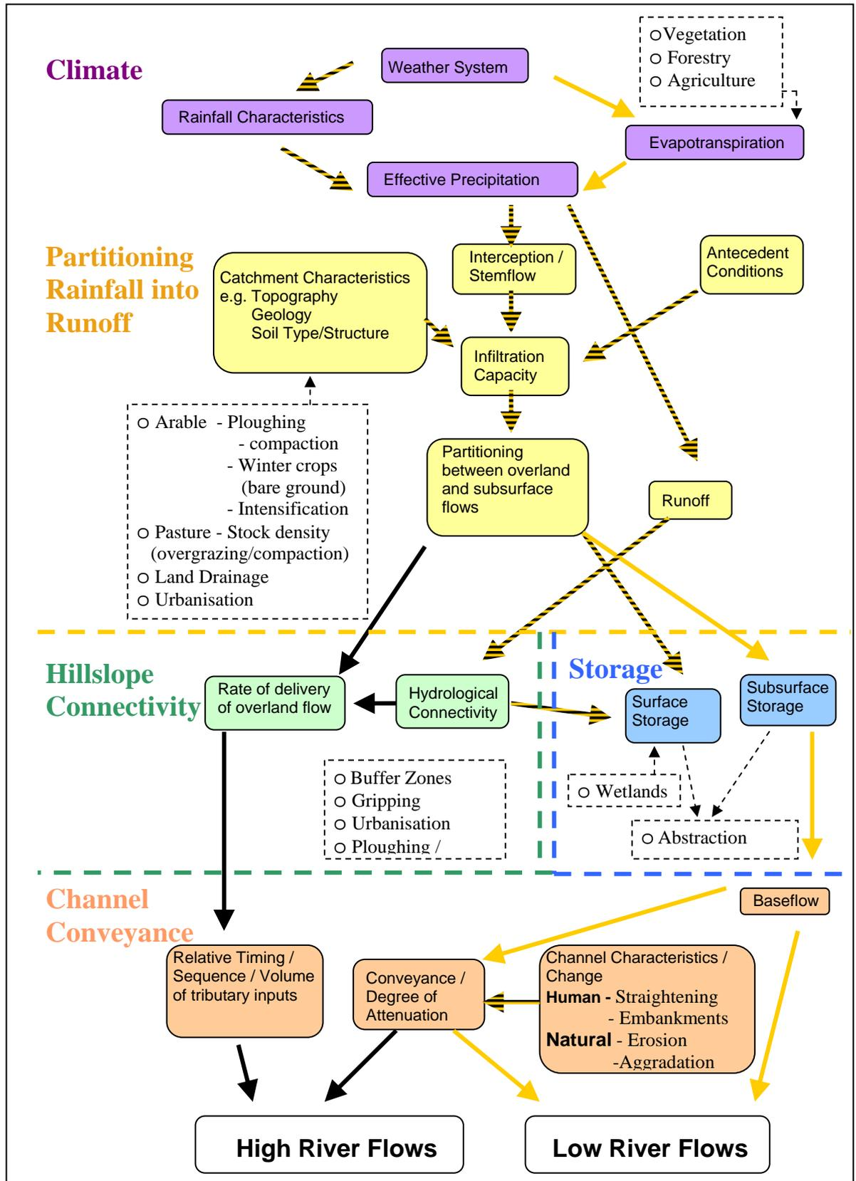
Figure 7.2 Conceptual framework based on hydrological process that results in high and low river flows.
