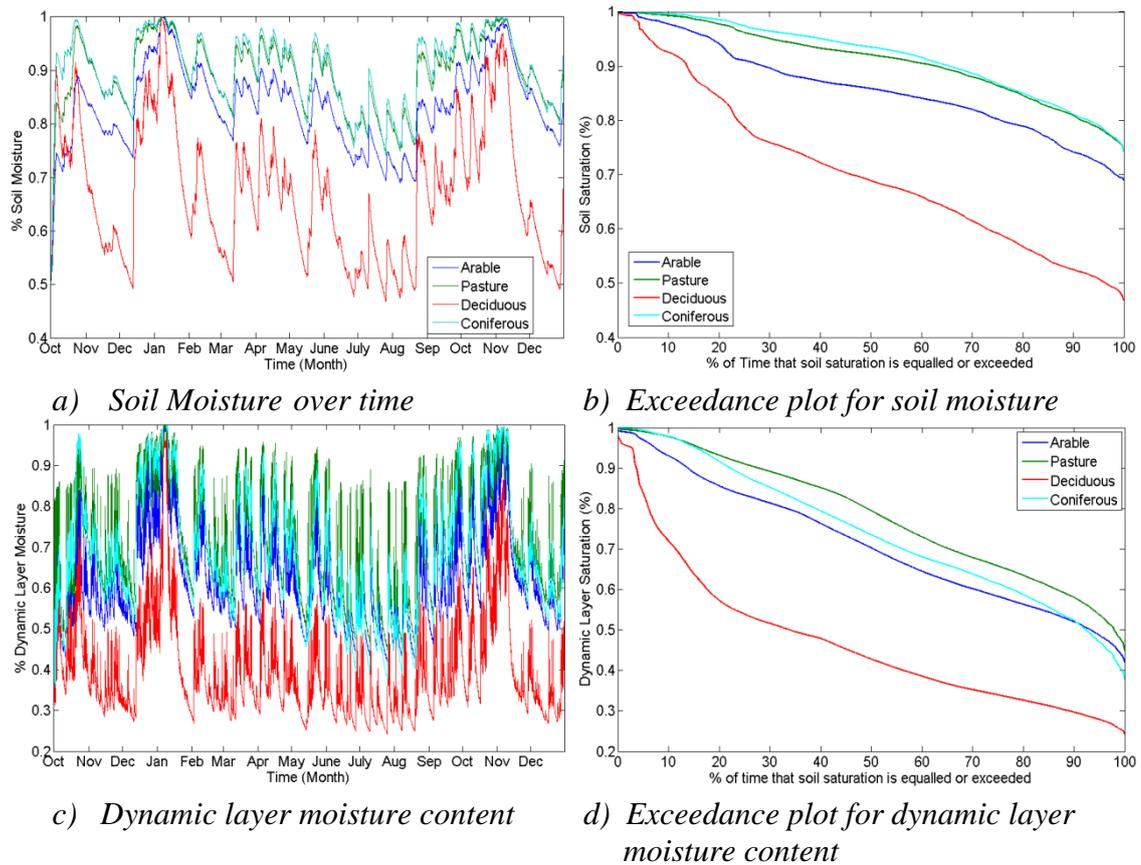
**Figure 9.19** Moisture content of the soil store, including both the main soil and dynamic layer.
