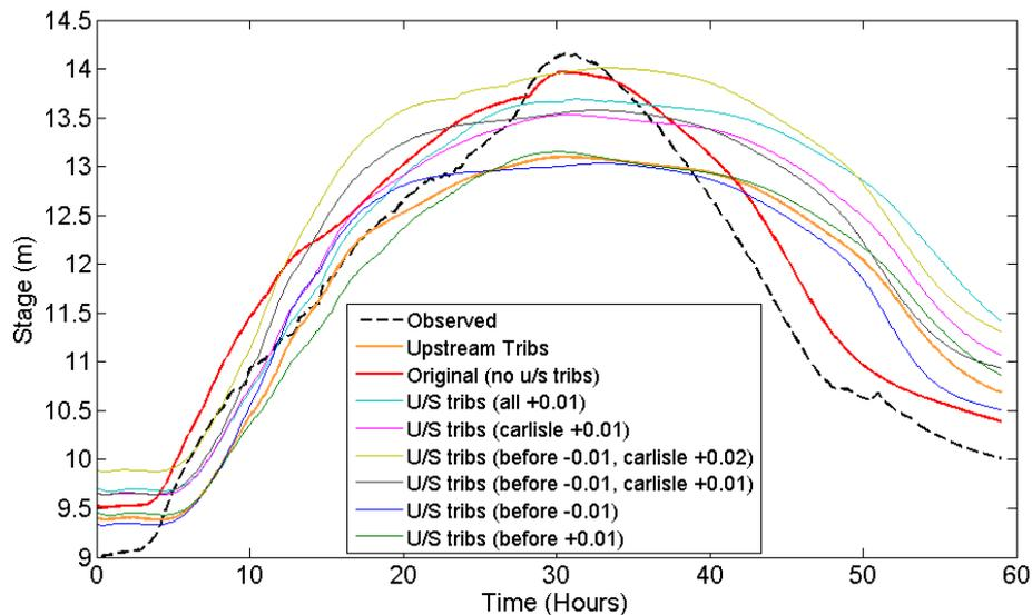
**Figure 5.4** Sensitivity analysis of Sheepmount hydrograph to Manning's  $n$ . Simulations represent changing Manning's  $n$  in different reaches of Eden. e.g. U/S tribs (before -0.01, Carlisle +0.01 = Manning's  $n$  decreased by 0.01 before Carlisle and increased by 0.01 in Carlisle itself).
