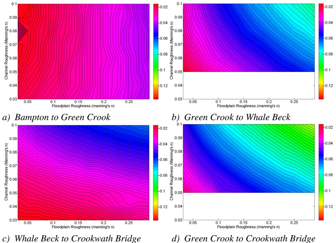
**Figure 9.36** Impact of roughness modification on sub-catchment scale (Askham) peak flow magnitude for the 10<sup>th</sup> January 2005 flood event. Units are Stage in metres, where negative values are decreases.
