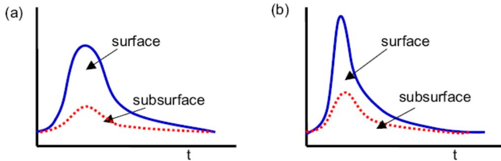
**Figure 2.4** Response of a hillslope to the same storm for a (a) pre-war landscape and (b) modern landscape, showing the partitioning of precipitation into surface and subsurface flows. (O’Connell *et al.*, 2004)
