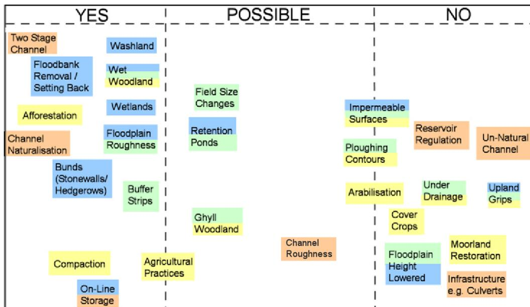
**Figure 7.4** Stakeholder prioritisation, including processes which scenario effects (colour coding relates to the hydrological process conceptual framework, with yellow representing partitioning rainfall into runoff, green representing hydrological connectivity, blue representing storage, and orange representing channel conveyance)
