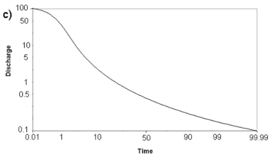
Figure 3.31c Flow Duration Curve – Normalised Probability scaled axes.
