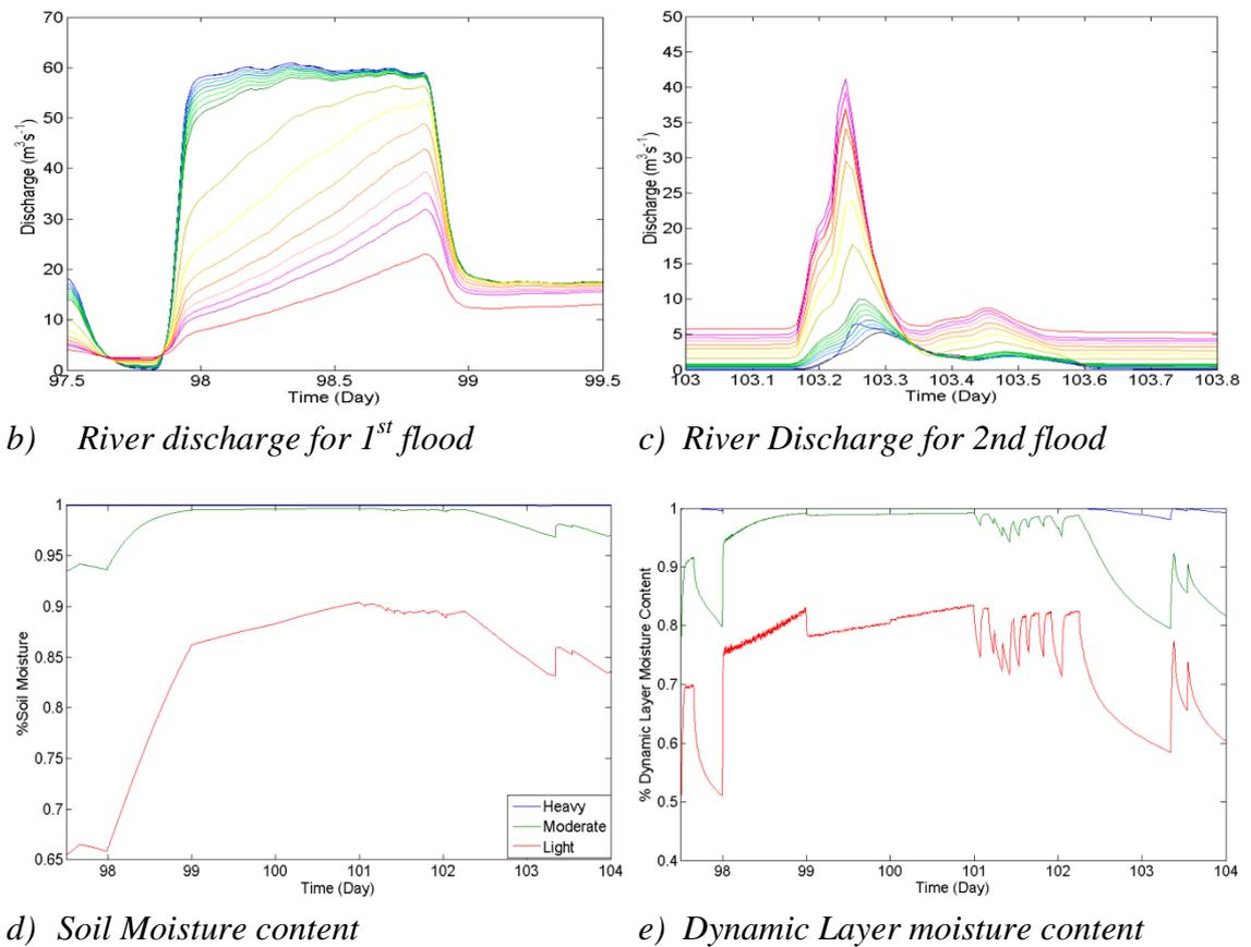
**Figure 9.13** River discharge and Soil moisture content for the continuum of compaction scenarios for the January 2005 flood
