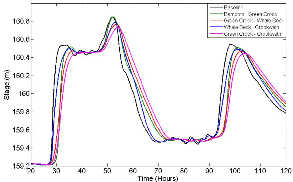
**Figure 9.38** Effect of the roughest scenario (channel 0.1, floodplain 0.29) for the four different reaches on stage hydrograph at Askham
