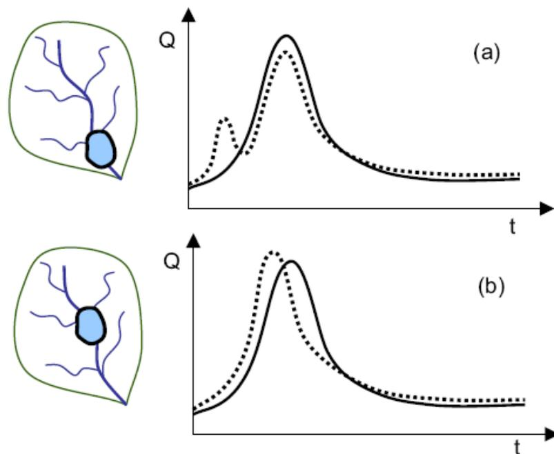
**Figure 1.1** Effect of land management change location upon the downstream flood hydrograph. (Blue area shows area of compacted soils, solid line indicates pre-change hydrograph, and dashed line shows post-change hydrograph). (O’Connell *et al.*, 2004)
