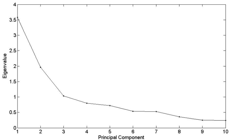
**Figure 6.10** Scree plot for principal components analysis
