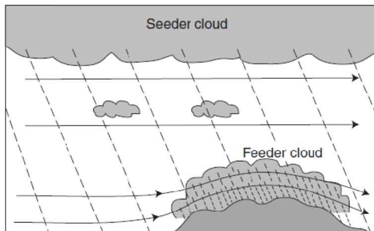
**Figure 4.8** A schematic of the seeder-feeder mechanism adapted (Roberts et al. 2009) from the *Forecasters Reference book* (Meteorological Office, 1997)
