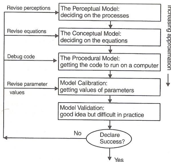
**Figure 2.1** Flow diagram of the modelling procedure (Beven, 2001).
