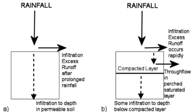
**Figure 2.3** Schematic showing the effects of compaction on soil infiltration (adapted from O’Connell *et al.*, 2004)
