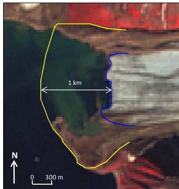
Figure 3.5: Glacier number 115 in the northwest study area, showing the terminus position in the LIA (yellow line, extrapolated from the latero-frontal moraine) and 1999 (blue line). Background image is Landsat ETM+ from the 24 th of July 1999, displayed using bands 4-3-2 (red, green, blue).
