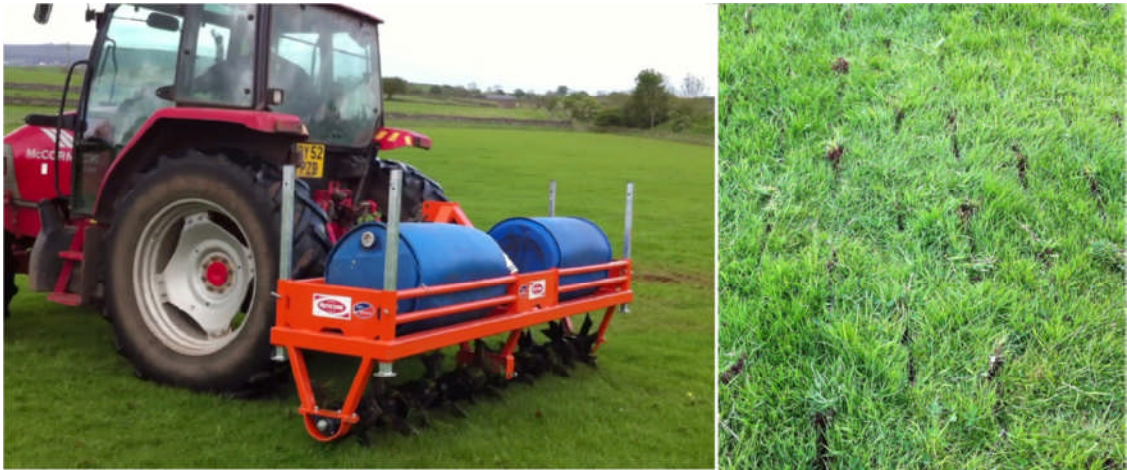
Figure 3.7 Photographs of the Ritchie Grassland Aerator© in use (left) and (right) the slits produced on the grassland surface immediately after aeration.
