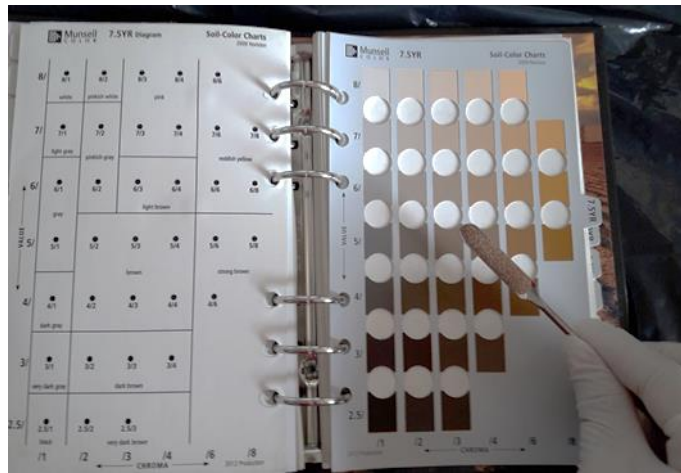
Figure 3.10: Matching the colour of a sediment sample against the standardised swatches for brown shades within the Munsell soil colour.
