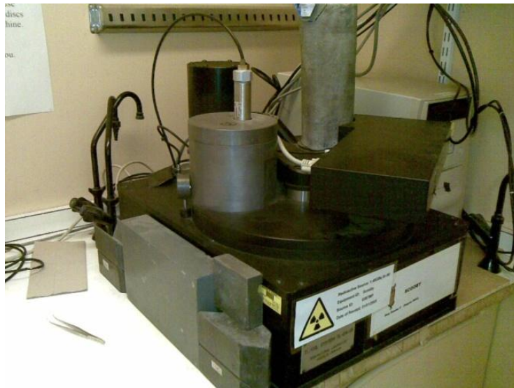
Figure 3.1: Luminescence measurements were made on TL-DA-15 fitted with a single grain attachment (Scooby).
