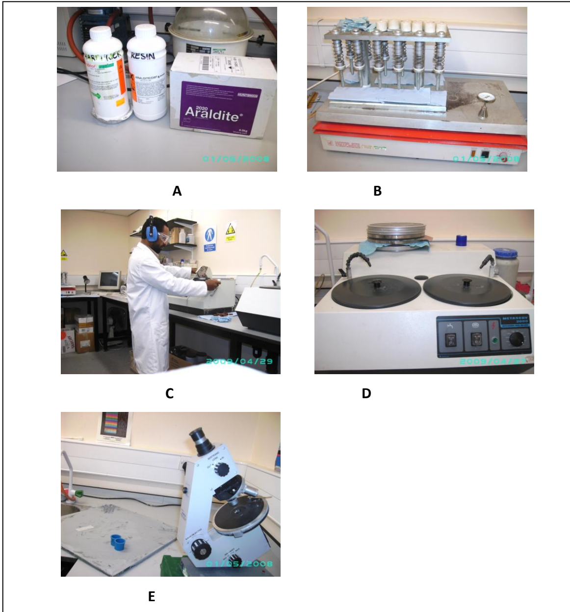
Figure 3.3: The stages of preparation for thin sections. (A) Araldite DBF resin and Araldite XD716 hardener used to impregnate the samples; (B) samples put on the hotplate to warm; (C) cutting the samples slowly for standard thin sections; (D) Metaserv 2000 grinder to grind down the samples; (E) glass slides ground down by hand on a flat glass using black silicon carbide 600 grit and checked under a low-powered microscope.
