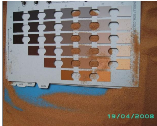
Figure 3.5: Examples of determining the colour by comparing the sand sample (e.g. QA .08.25E)
