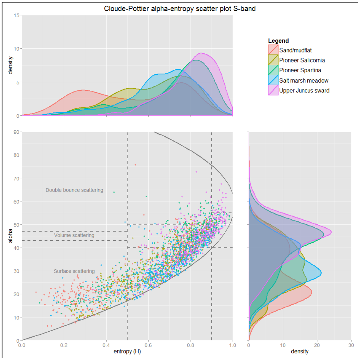
Figure 23 – Scatter plots and density plots of \alpha against H for S-band SAR data.
