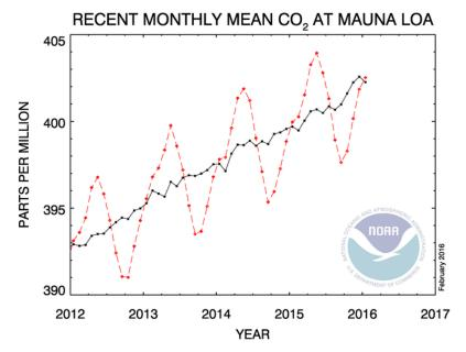
**Figure 1.1.** The graph shows recent monthly mean CO<sub>2</sub> measured at Mauna Loa Observatory, Hawaii. The dashed red line represents the monthly mean values, centered on the middle of each month while black line represents the same, after correction for the average of 7 adjacent seasonal cycles. Image reproduced with copyright permission from the Scripps Institution of Oceanography.
