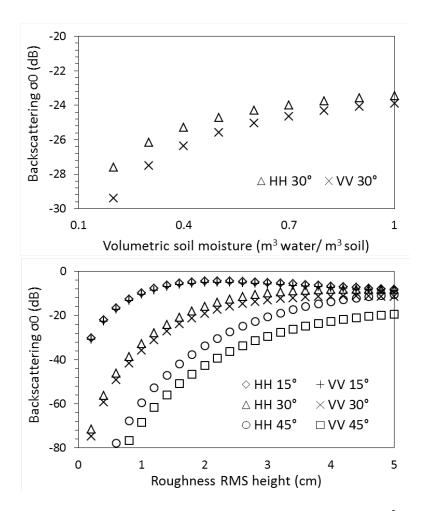
Figure 4.1. S-band ground backscatter vs. soil volumetric moisture (m<sup>3</sup> water/m<sup>3</sup> soil) (top) and soil RMS height (cm) (bottom) for co-polarisation at 15°, 30° and 45° radar incidence range.
