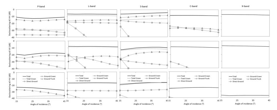
Figure 4.7. Total co- and cross-polarisations canopy backscatter components vs. scattering angle from 830 leaves and 4.1 branch density Birch at fourth branch levels for P-, L-, S-, C and X-band.
