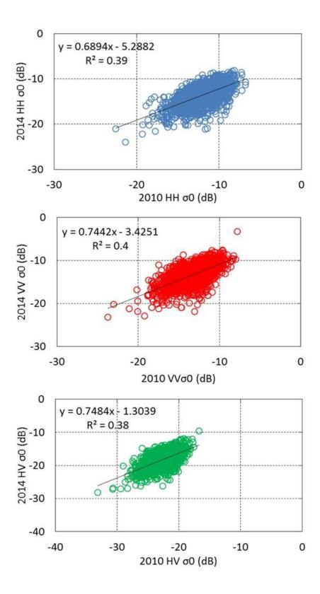
Figure 3.9. S-band backscatter comparison for forest (2640 ancient tree points) class between re-scaled 2010 and 2014 SAR imageries.
