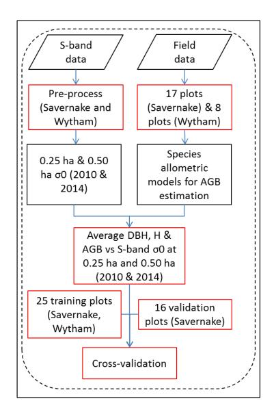
**Figure 3.12.** Methodology flowchart for forest biophysical retrieval \* DBH: tree diameter at breast height, H: canopy height and  $\sigma$ 0: backscatter sigma-nought.
