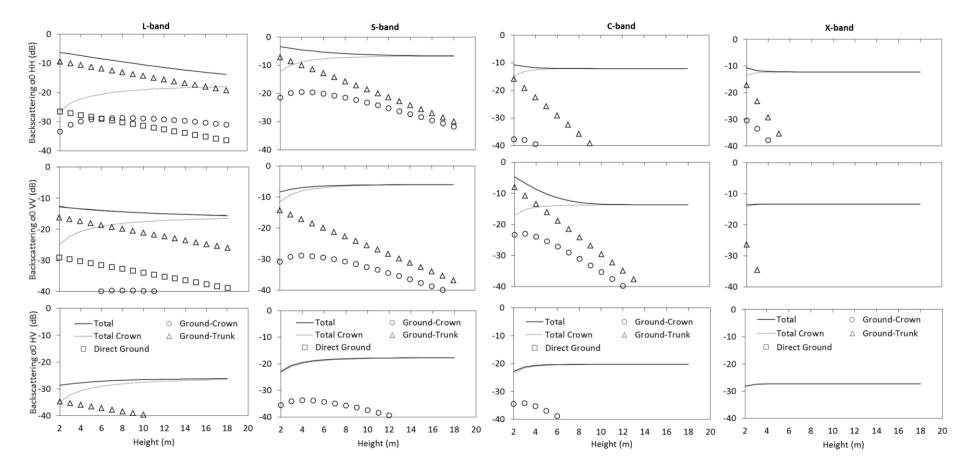
Figure 4.9. Total co- and cross-polarisations canopy backscatter components vs. canopy stand height (m) from 830 leaves and 4.1 branch density Birch for L-, S-, C- and X-band at 30° incidence angle.
