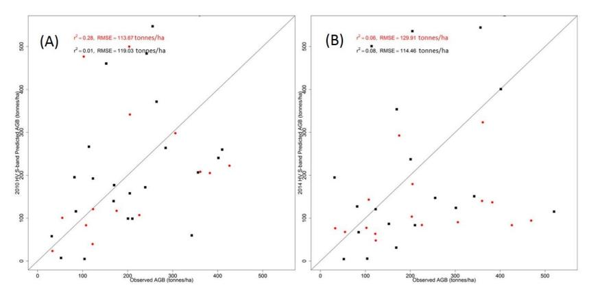
**Figure 6.12.** Results of biomass estimation using S-band backscatter (σ0) based on training stands (25 stands-black square) and validation stands (16 stands- red circle) for HV-polarisation at 0.25 ha for 2010 (A) and 2014 (B). Locations of training and validation stands for Savernake are shown in Figure 6.1.
