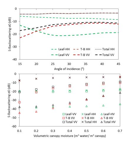
**Figure 4.5.** S-band backscatter vs. canopy parts at 0.5 volumetric moisture (m<sup>3</sup> water/m<sup>3</sup> canopy) across incidence angles (top) and at varying volumetric moisture (m<sup>3</sup> water/m<sup>3</sup> canopy) at 30° radar range (bottom) where T- and B- represents trunk and branches respectively.
