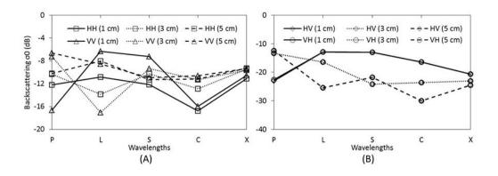
**Figure 4.13.** Total canopy backscatter vs. frequency from 85,000 needles and 3.4 branch density per cubic meter at varying branch sizes (1 cm, 3 cm, 5 cm) for co- (A) and cross-polarisations (B) Norway spruce at 30° scattering angle.
