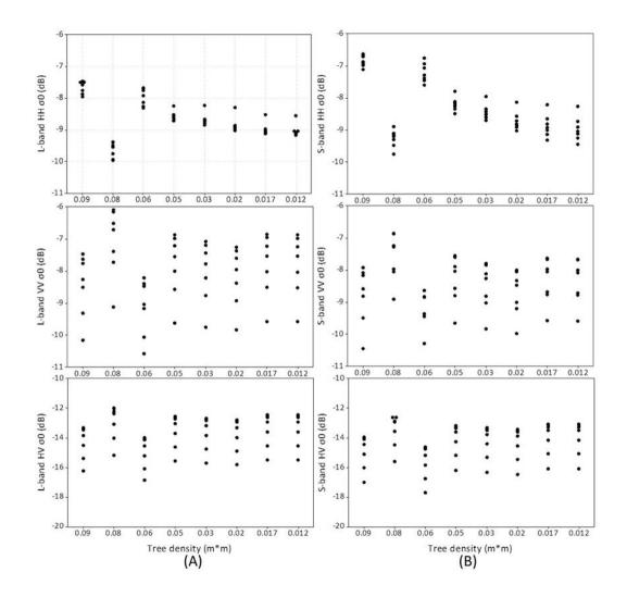
**Figure 4.16.** Simulated backscatter for forest degradation as a function of tree density with varying canopy height, DBH and AGB for L- (A) and S-band (B) (15° -45° incidence angles).
