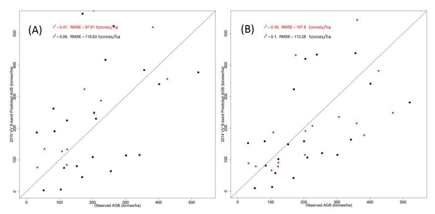
**Figure 6.11.** Results of biomass estimation using S-band backscatter (σ0) based on training stands (25 stands-black square) and validation stands (16 stands- red circle) for VV-polarisation at 0.25 ha for 2010 (A) and 2014 (B). Locations of training and validation stands for Savernake are shown in Figure 6.1.
