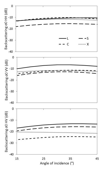
**Figure 4.11.** Total co-polarisation (top, middle) and cross-polarisation (bottom) canopy backscatter vs. scattering angle from 85,000 needles and 3.4 branch density Norway spruce for L-, S-, C- and X-band.
