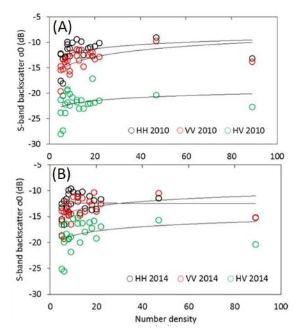
Figure 6.6. Stand number density relationship with S-band backscatter ( $\sigma$ 0) at 0.25 ha for 2010 (A) and 2014 (B).
