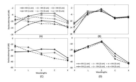
**Figure 4.8.** Total canopy backscatter vs. SAR wavelengths from 4.1 branches per cubic meter, primary branch diameter (1 cm, 3 cm, 5 cm) (A, C) with 830 leaves per cubic meter (B, D) Birch stand at 30° scattering angle for co- and cross-polarisations.
