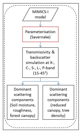
Figure 3.6. Methodology flowchart for MIMICS-I modelling.
