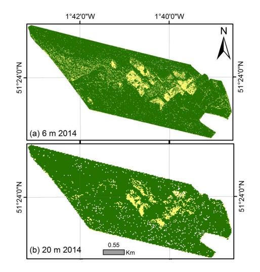
**Figure 5.3.** F/NF cover map of Savernake using S-band polarimetry and maximum likelihood algorithm at 6 m (a) and 20 m (b) resolutions.
