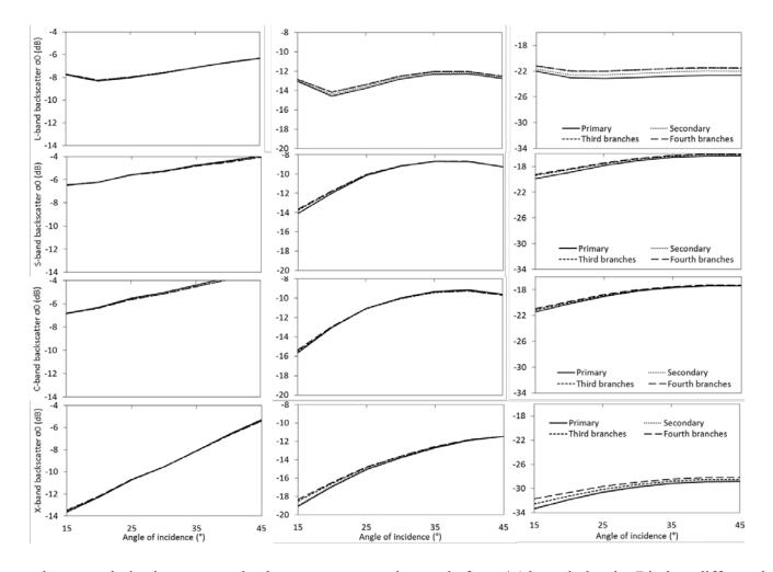
Figure 4.4. Total co- and cross-polarisations canopy backscatter vs. scattering angle from 4.1 branch density Birch at different branch levels for L-, S-, C- and X-band.
