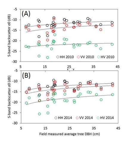
Figure 6.7. Average tree diameter relationship with S-band backscatter ( $\sigma$ 0) at 0.25 ha for 2010 (A) and 2014 (B).
