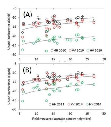
Figure 6.5. Average canopy height relationship with S-band backscatter ( $\sigma$ 0) at 0.25 ha for 2010 (A) and 2014 (B).
