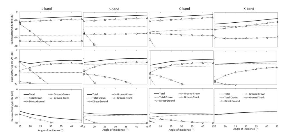
Figure 4.6. Total co-and cross-polarisations canopy backscatter components vs. scattering angle from 830 leaves and 4.1 branch density Birch at primary branch level for L-, S-, C- and X-band.
