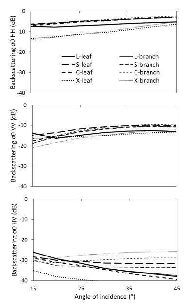
**Figure 4.3.** Total co- and cross-polarisations canopy backscatter vs. scattering angle from 830 leaves and 4.1 branch density Birch for L-, S-, C- and X-band.
