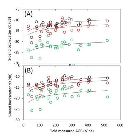
Figure 6.8. Above-ground biomass relationship with S-band backscatter ( $\sigma$ 0) for 2010 (A) and 2014 (B).
