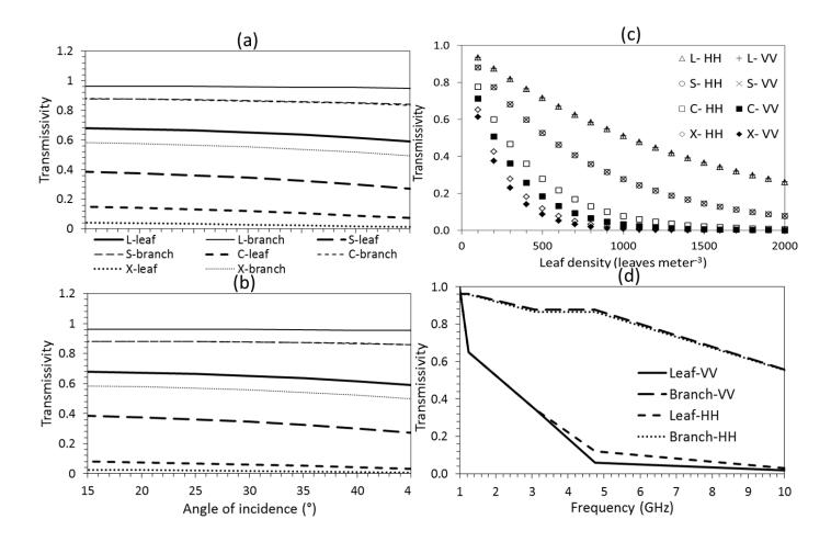
**Figure 4.2.** HH (a) and VV (b) polarisations crown transmissivity vs. scattering angle from 830 leaves per cubic meter and 4.1 branches per cubic meter, crown transmissivity vs. density of leaves at 30° scattering angle (c) and crown transmissivity vs. frequency for Birch for L-, S-, C- and X-bands (d).
