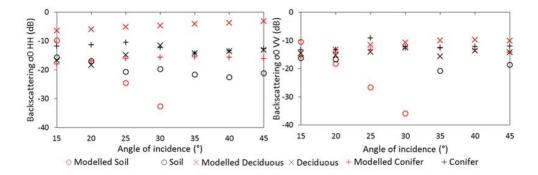
Figure 4.14. Simulated forest canopy (deciduous, conifers) and soil total backscatter relationship as a function of radar incidence range at S-band (modelled against SAR data).
