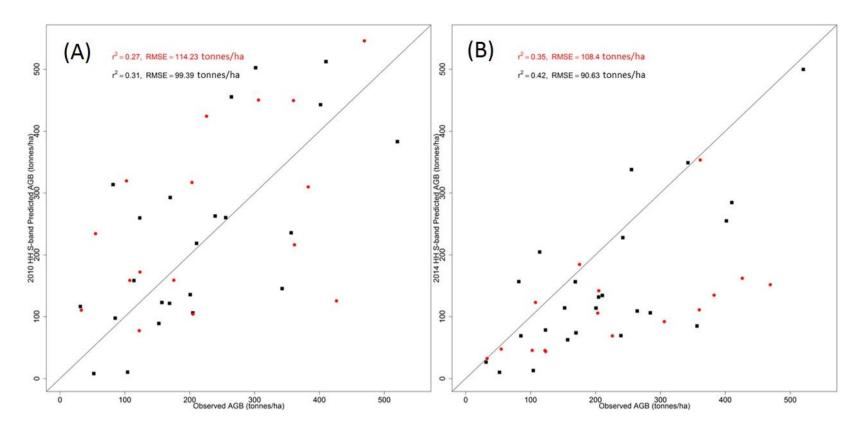
**Figure 6.10.** Results of biomass estimation using S-band backscatter (σ0) based on training stands (25 stands-black square) and validation stands (16 stands- red circle) for HH-polarisation at 0.25 ha for 2010 (A) and 2014 (B). Locations of training and validation stands for Savernake are shown in Figure 6.1.
