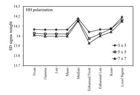
Figure 3.2. Comparison of different adaptive filters at different kernels (2014 acquired HH-polarisation in Savernake forest).
