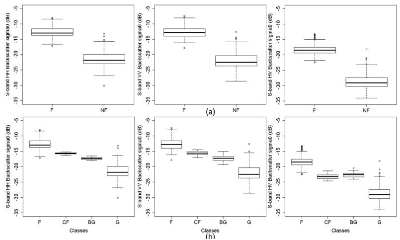
Figure 5.2. Box-plots of scattering returns of S-band SAR backscatter in 105 (F- Forest) and105 (NF- Non-forest) sample plots (a) and different non-forest types with 50 (CF- Cleared-felled), 45 (BG- Bare-ground) and 10 (G- Grassland) sample plots (b). The central box in each box plot shows the inter-quartile range and median; whiskers indicate the 10th and 90th percentiles.
