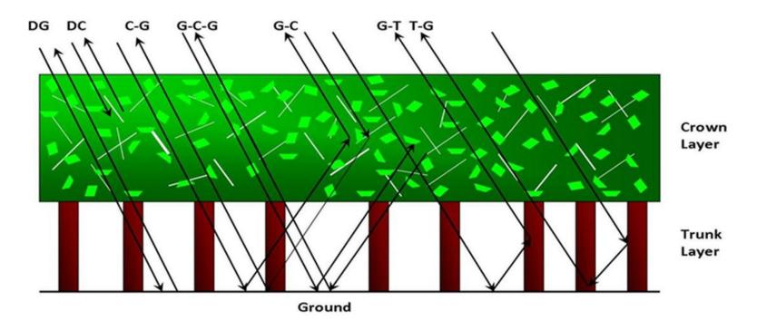
Figure 2.1. Overview of MIMICS model structure with different interaction components (DG-direct ground, DC-direct crown, C-G-crownground, G-C-G- ground-crown-ground, GC-ground crown, G-T or T-G-ground/trunk) from forest canopies (Ulaby et al. 1990). Image reproduced with copyright permission from the Radiation Laboratory, University of Michigan.
