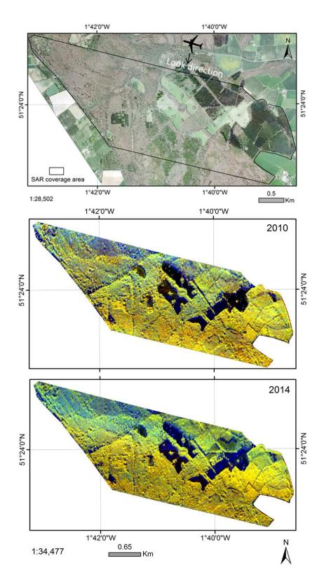
**Figure 3.11.** Aerial photo (top) and 6 m S-band SAR data acquired in 2010 (middle) and 2014 (bottom) over Savernake forest as HH-, VV- backscatter and
