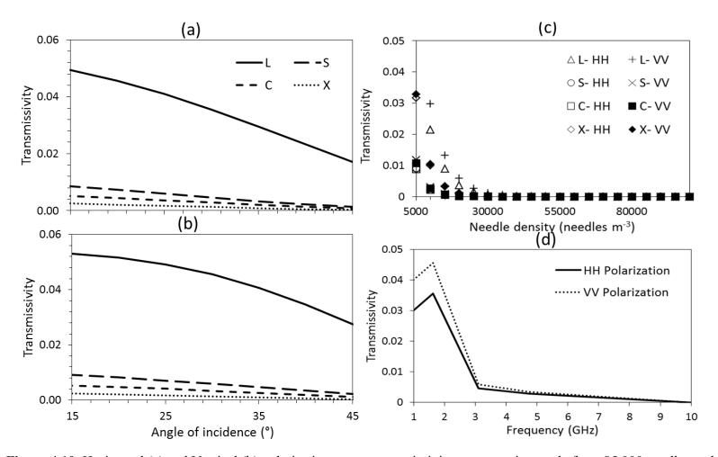
**Figure 4.10.** Horizontal (a) and Vertical (b) polarisation crown transmissivity vs. scattering angle from 85,000 needles and 3.4 branches per cubic meter Norway spruce, needle density at 30° scattering angle (c) and versus frequency at 30° scattering angle for L-, S-, C- and X-band.
