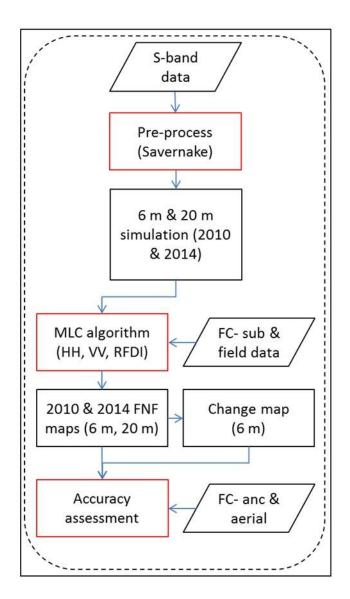
Figure 3.8. Methodology flowchart for mapping forest/ non-forest and change detection. \*MLC: maximum likelihood classification, RFDI: Radar Forest Degradation Index, FC- sub/ - anc: Forestry Commission sub-compartment/ ancient database.
