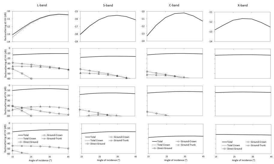
Figure 4.12. Total co-and cross-polarisations canopy backscatter components vs. scattering angle from needle-branch canopy layer 85,000
