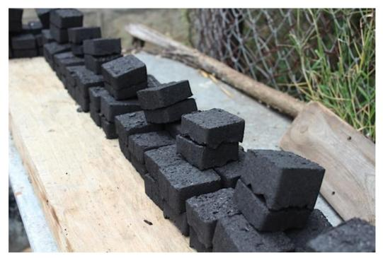
Fig. 6.4. Carbonized papyrus briquettes (cuboid type) ready to be used (photo: V. Lafford).
