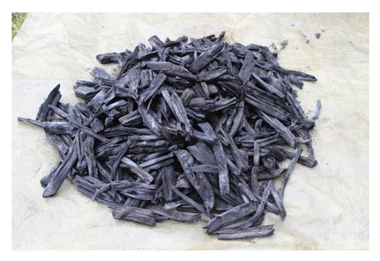
Fig. 3.8. Carbonized papyrus fines ready to be crushed and mixed with binding agent (photo: V. Lafford).
